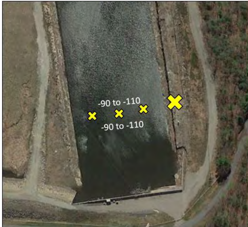
Figure A-18. The Upper Reservoir monitoring station consisting of an Orion receiver with double 3-element Yagi (location indicated by large X) and three, in-water dropper antennas (location indicated by small x) that were suspended mid-depth using 8-lb. downrigger weights. The test tag produced power levels ranging from -110 to -90 dB.
