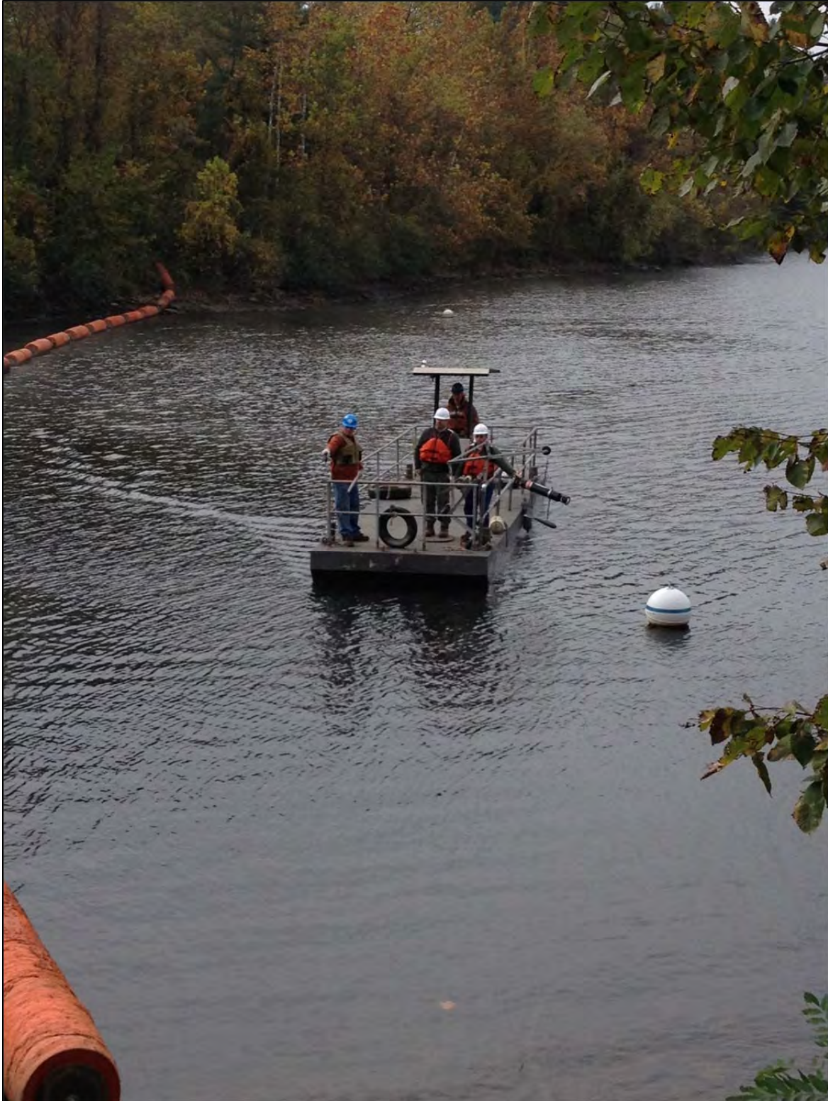
Figure 3.4: Configuration of the LISST-100x during sampling at the Northfield Mountain Tailrace with a small barge.
