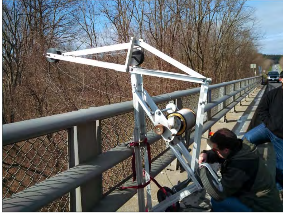
Figure 3.5: Crane system used to lower the LISST-100x from the Route 10 Bridge.
