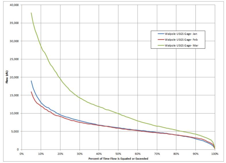
Figure 3.3.2.1.1-3: Connecticut River at Walpole, NH, Jan, Feb and Mar Flow Duration Curve, Mar 1942-Dec 2014, Drainage Area = 5,493 mi<sup>2</sup>
