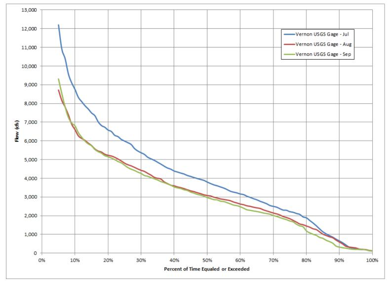
Figure 3.3.2.1.1-10: Connecticut River below Vernon Dam, VT, Jul, Aug and Sep Flow Duration Curve, Oct 1944-Sep 1973, Drainage Area = 6,266 mi<sup>2</sup>
