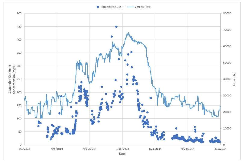
Figure 3.3.1.1.4-2: 2014 Spring Freshet – SSC vs. Flow<sup>26</sup>
