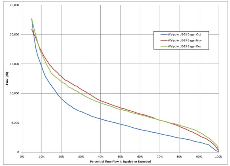
Figure 3.3.2.1.1-6: Connecticut River at Walpole, NH, Oct, Nov, and Dec Flow Duration Curve, Mar 1942-Dec 2014, Drainage Area = 5,493 mi<sup>2</sup>
