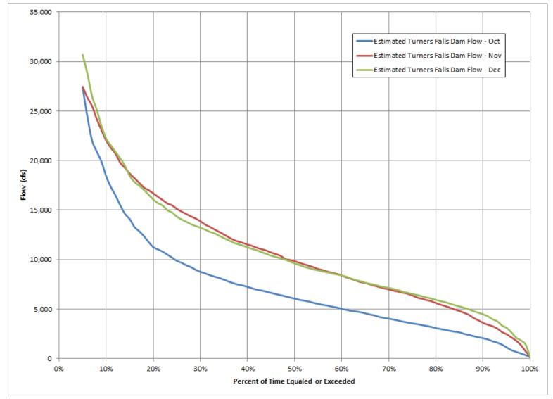
Figure 3.3.2.1.1-21: Connecticut River at Turners Falls Dam, Oct, Nov and Dec Flow Duration Curve, Jan 1941-Dec 2014, Drainage Area= 7,860 mi<sup>2</sup>
