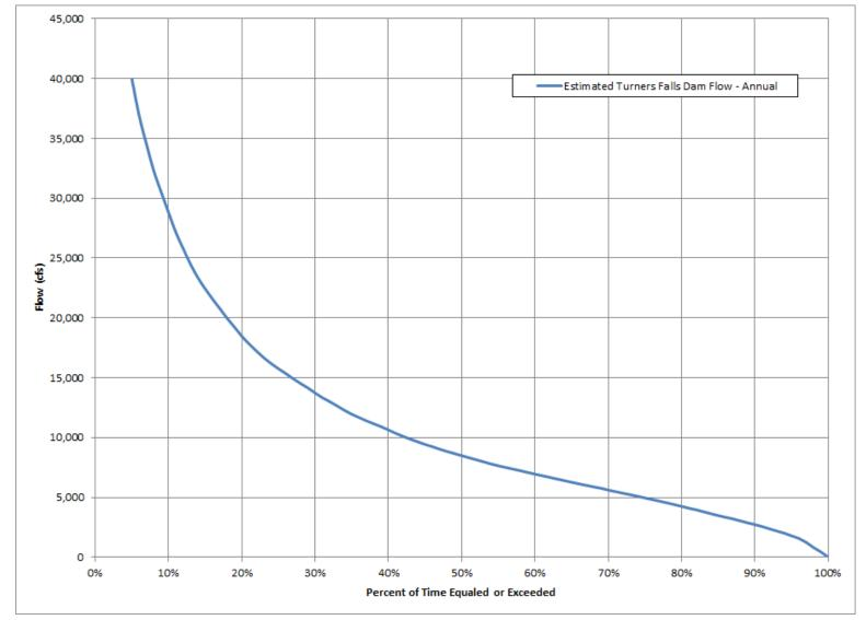
Figure 3.3.2.1.1-17: Connecticut River at Turners Falls Dam, Annual Flow Duration Curve, Jan 1941-Dec 2014, Drainage Area= 7,860 mi<sup>2</sup>
