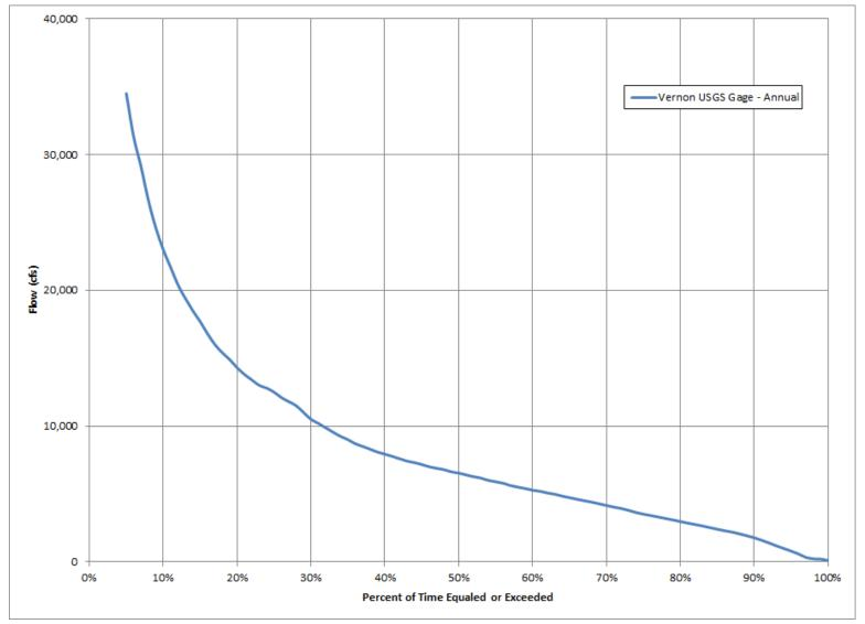
Figure 3.3.2.1.1-7: Connecticut River below Vernon Dam, VT, Annual Flow Duration Curve, Oct 1944-Sep 1973, Drainage Area= 6,266 mi<sup>2</sup>
