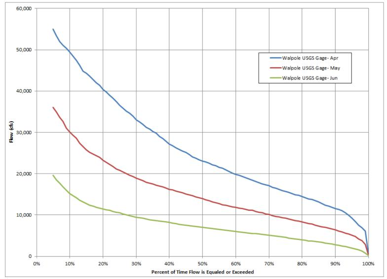
Figure 3.3.2.1.1-4: Connecticut River at Walpole, NH, Apr, May and Jun Flow Duration Curve, Mar 1942-Dec 2014, Drainage Area= 5,493 mi<sup>2</sup>
