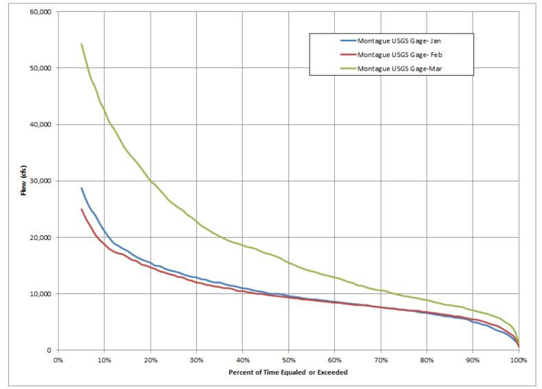
Figure 3.3.2.1.1-13: Connecticut River at Montague, MA, Jan, Feb and Mar Flow Duration Curve, Apr 1940-Dec 2014, Drainage Area= 7,860 mi<sup>2</sup>
