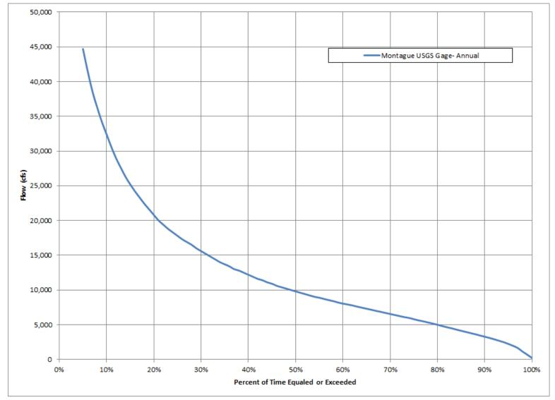
Figure 3.3.2.1.1-12: Connecticut River at Montague, MA, Annual Flow Duration Curve, Apr 1940-Dec 2014, Drainage Area= 7,860 mi<sup>2</sup>
