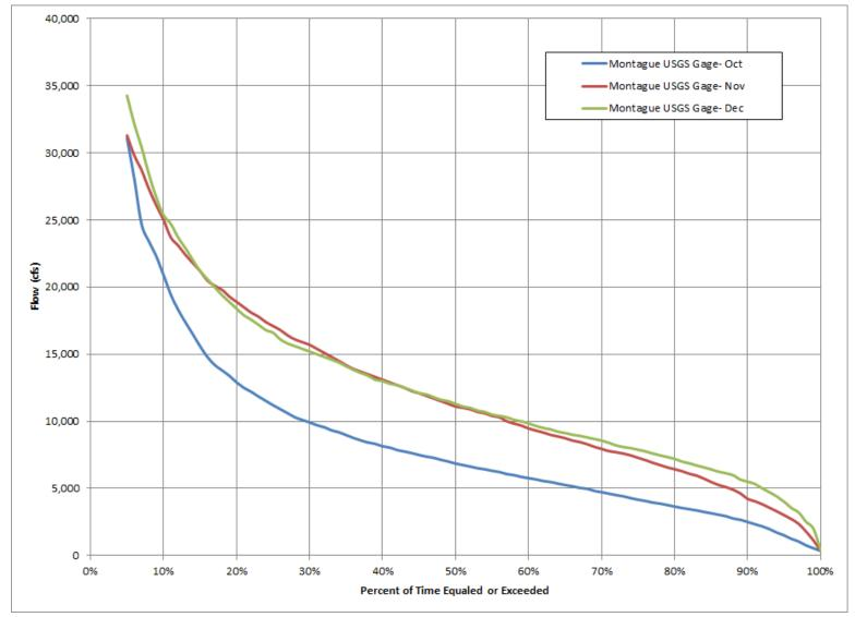
Figure 3.3.2.1.1-16: Connecticut River at Montague, MA, Oct, Nov and Dec Flow Duration Curve, Apr 1940-Dec 2014, Drainage Area= 7,860 mi<sup>2</sup>
