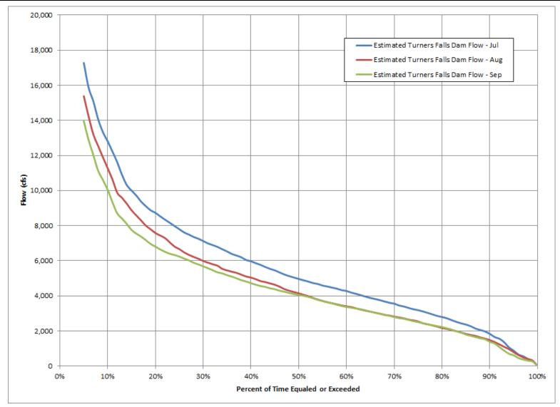
Figure 3.3.2.1.1-20: Connecticut River at Turners Falls Dam, Jul, Aug and Sep Flow Duration Curve, Jan 1941-Dec 2014, Drainage Area= 7,860 mi<sup>2</sup>
