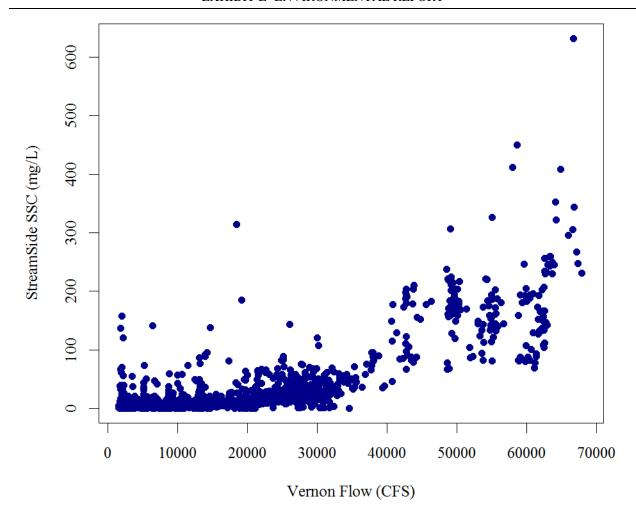
Figure 3.3.1.1.4-1: Connecticut River SSC vs. Vernon Discharge (2013-2015)<sup>25</sup>
