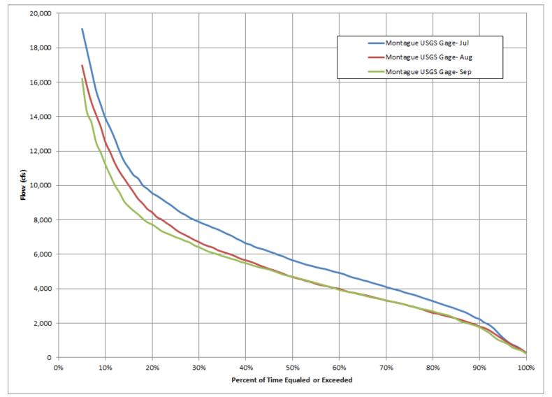
Figure 3.3.2.1.1-15: Connecticut River at Montague, MA, Jul, Aug and Sep Flow Duration Curve, Apr 1940-Dec 2014, Drainage Area= 7,860 mi<sup>2</sup>
