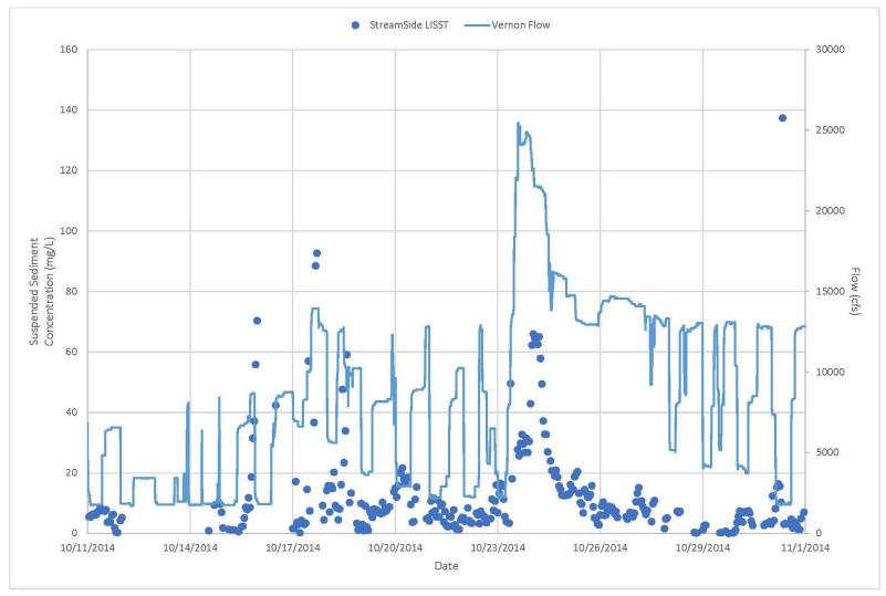
Figure 3.3.1.1.4-4: Typical Fall Period – SSC vs. Flow<sup>28</sup>
