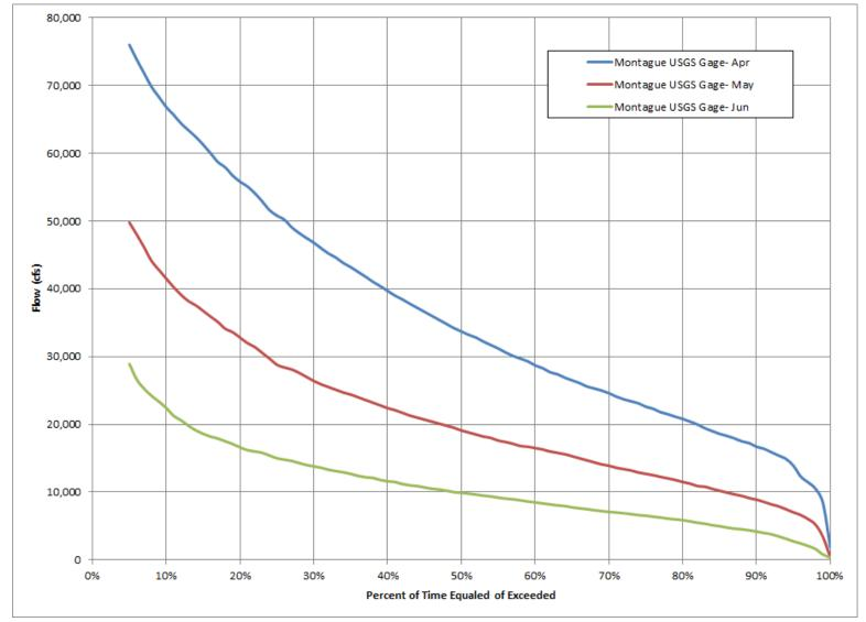
Figure 3.3.2.1.1-14: Connecticut River at Montague, MA, Apr, May and Jun Annual Flow Duration Curve, Apr 1940-Dec 2014, Drainage Area= 7,860 mi<sup>2</sup>
