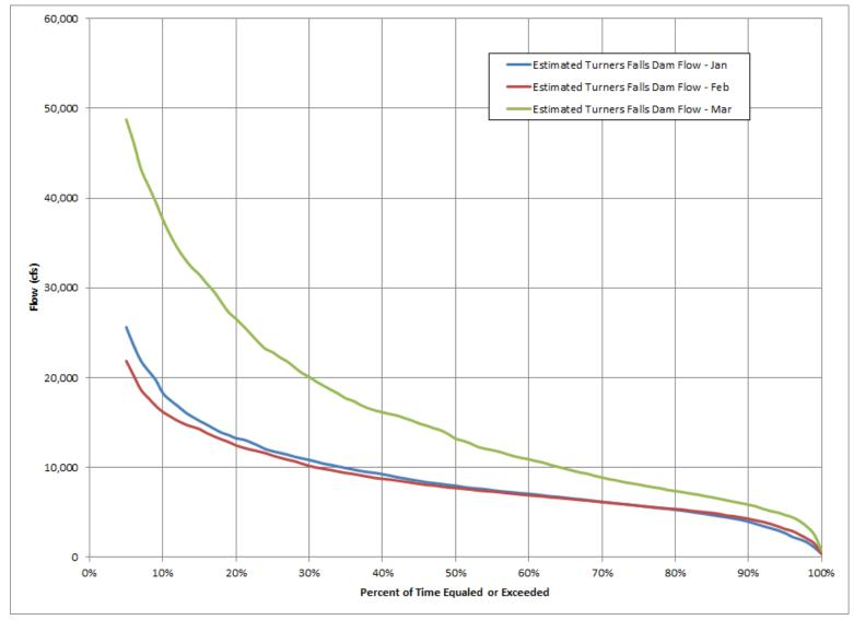
Figure 3.3.2.1.1-18: Connecticut River at Turners Falls Dam, Jan, Feb and Mar Flow Duration Curve, Jan 1941-Dec 2014, Drainage Area= 7,860 mi<sup>2</sup>
