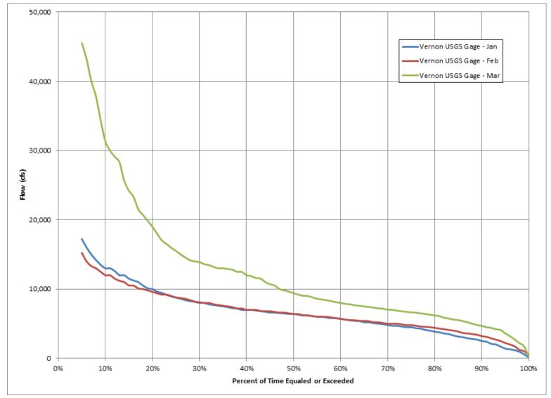
Figure 3.3.2.1.1-8: Connecticut River below Vernon Dam, VT, Jan, Feb and Mar Flow Duration Curve, Oct 1944-Sep 1973, Drainage Area= 6,266 mi<sup>2</sup>
