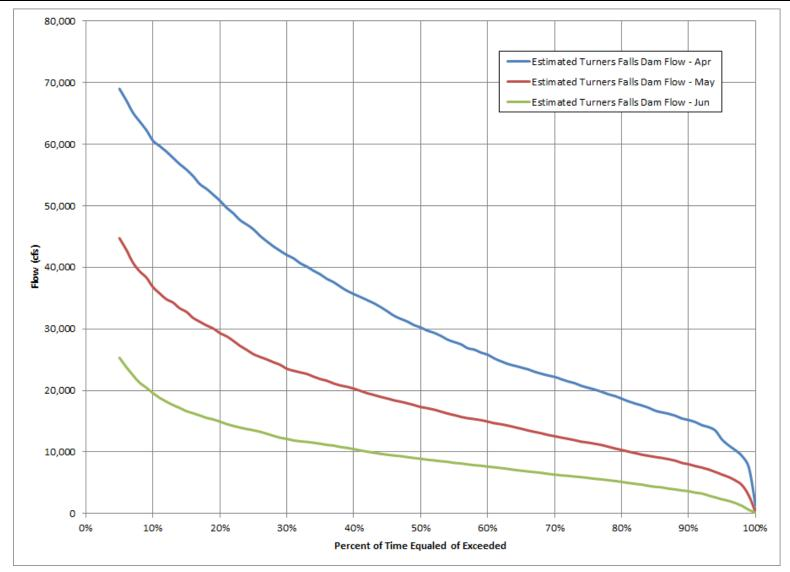
Figure 3.3.2.1.1-19: Connecticut River at Turners Falls Dam, Apr, May and Jun Annual Flow Duration Curve, Jan 1941-Dec 2014, Drainage Area= 7,860 mi<sup>2</sup>
