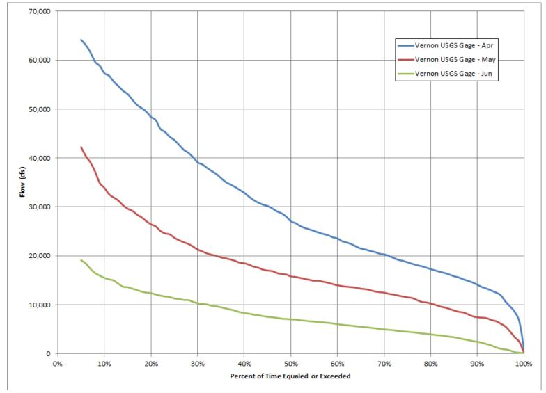
Figure 3.3.2.1.1-9: Connecticut River below Vernon Dam, VT, Apr, May and Jun Flow Duration Curve, Oct 1944-Sep 1973, Drainage Area= 6,266 mi<sup>2</sup>
