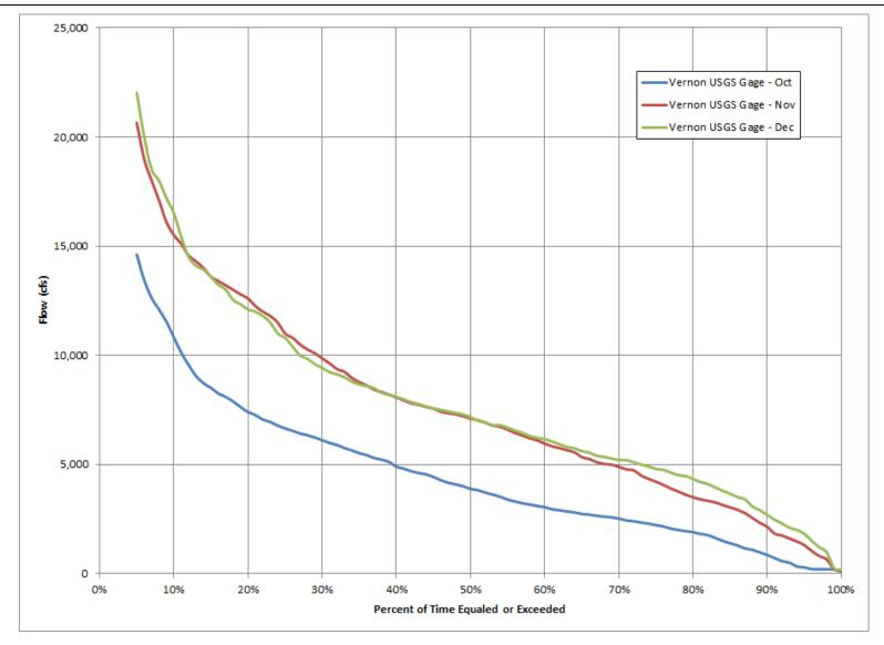
Figure 3.3.2.1.1-11: Connecticut River below Vernon Dam, VT, Oct, Nov and Dec Flow Duration Curve, Oct 1944-Sep 1973, Drainage Area= 6,266 mi<sup>2</sup>
