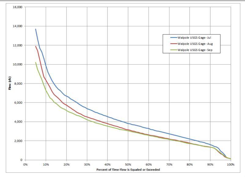
Figure 3.3.2.1.1-5: Connecticut River at Walpole, NH, Jul, Aug and Sep Flow Duration Curve, Mar 1942-Dec 2014, Drainage Area = 5,493 mi<sup>2</sup>
