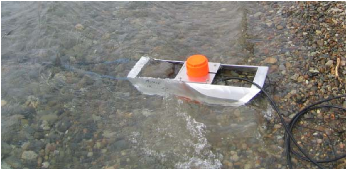
Figure 8. Up-looking transducer mounted on sled.
