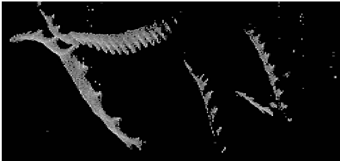
Figure 16. Echogram of acoustic imaging data showing the pronounced tail beat pattern (“caterpillar legs”) associated with the anguilliform swimming motion of eels. The echogram represents echo intensity over time (x-axis) and range (y-axis).
