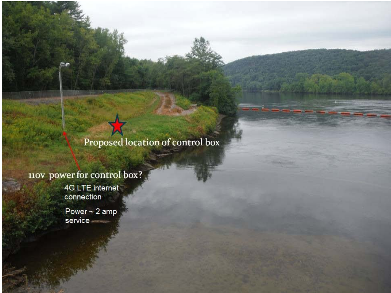
Figure 13. Pump-back-intake of the Northfield Mountain Pumped Storage facility. The star marks the proposed location of the weatherproof housing for the GPT that controls the acoustic monitoring system.
