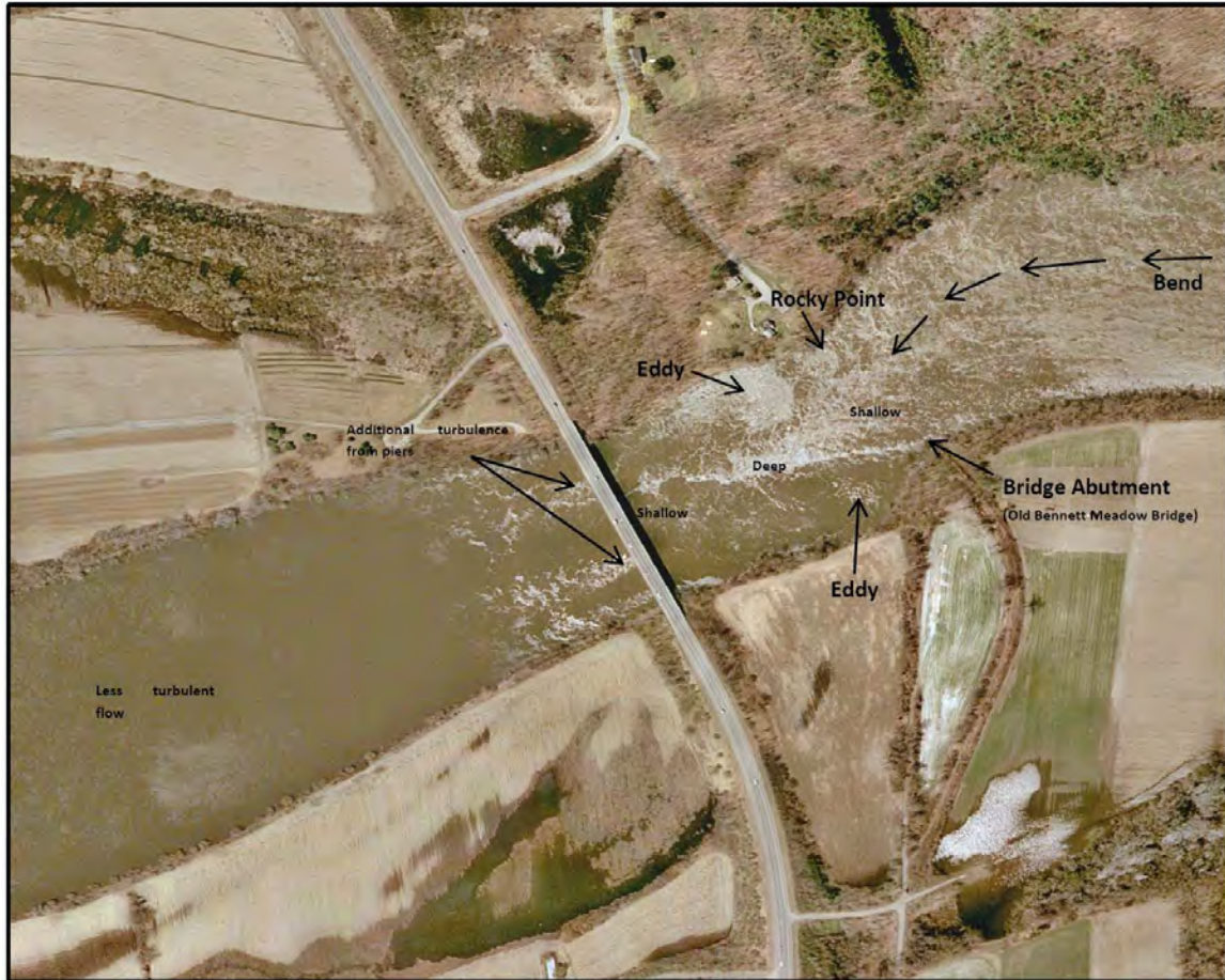
Figure 9. Flow characteristics in the vicinity of the Route 10 Bridge
