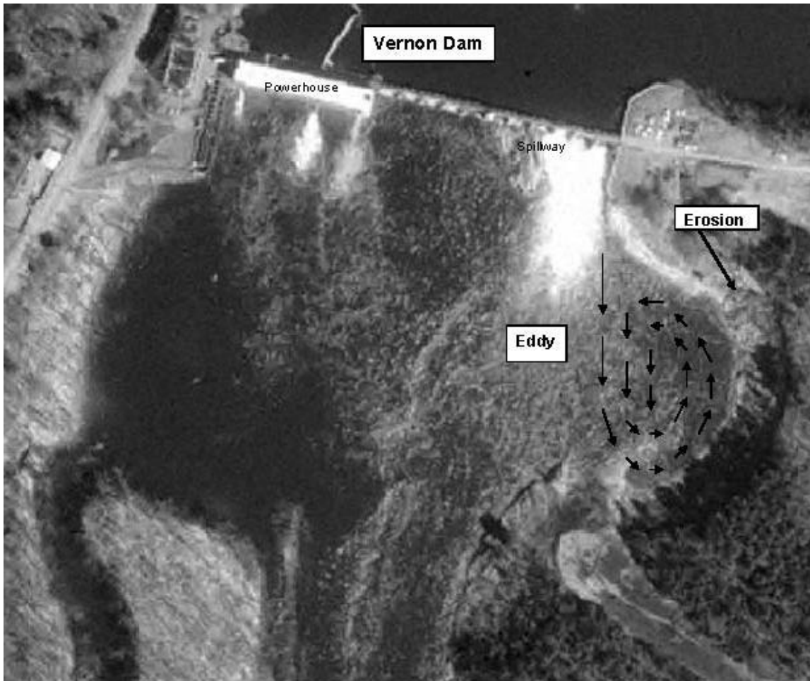
Figure 13. Eddy-induced erosion downstream of Vernon Dam
