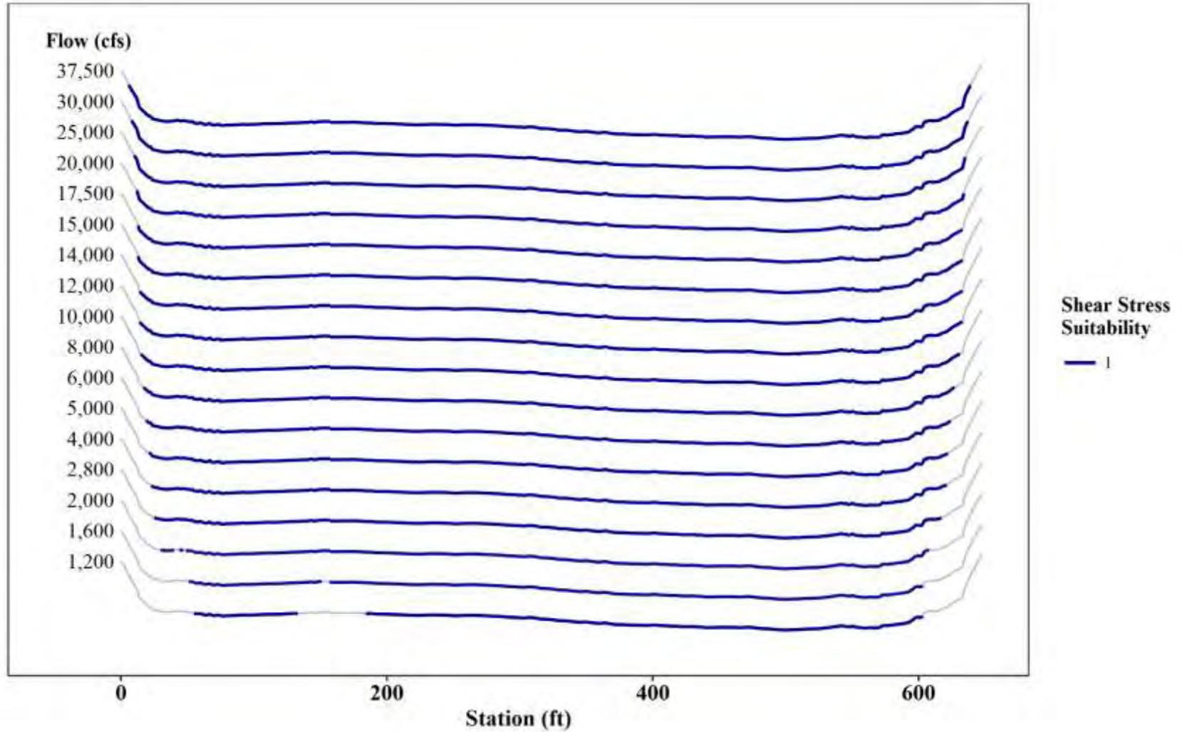
Figure 3.3-11: Shear Stress Mapping at T95 – Adult Yellow Lampmussel
