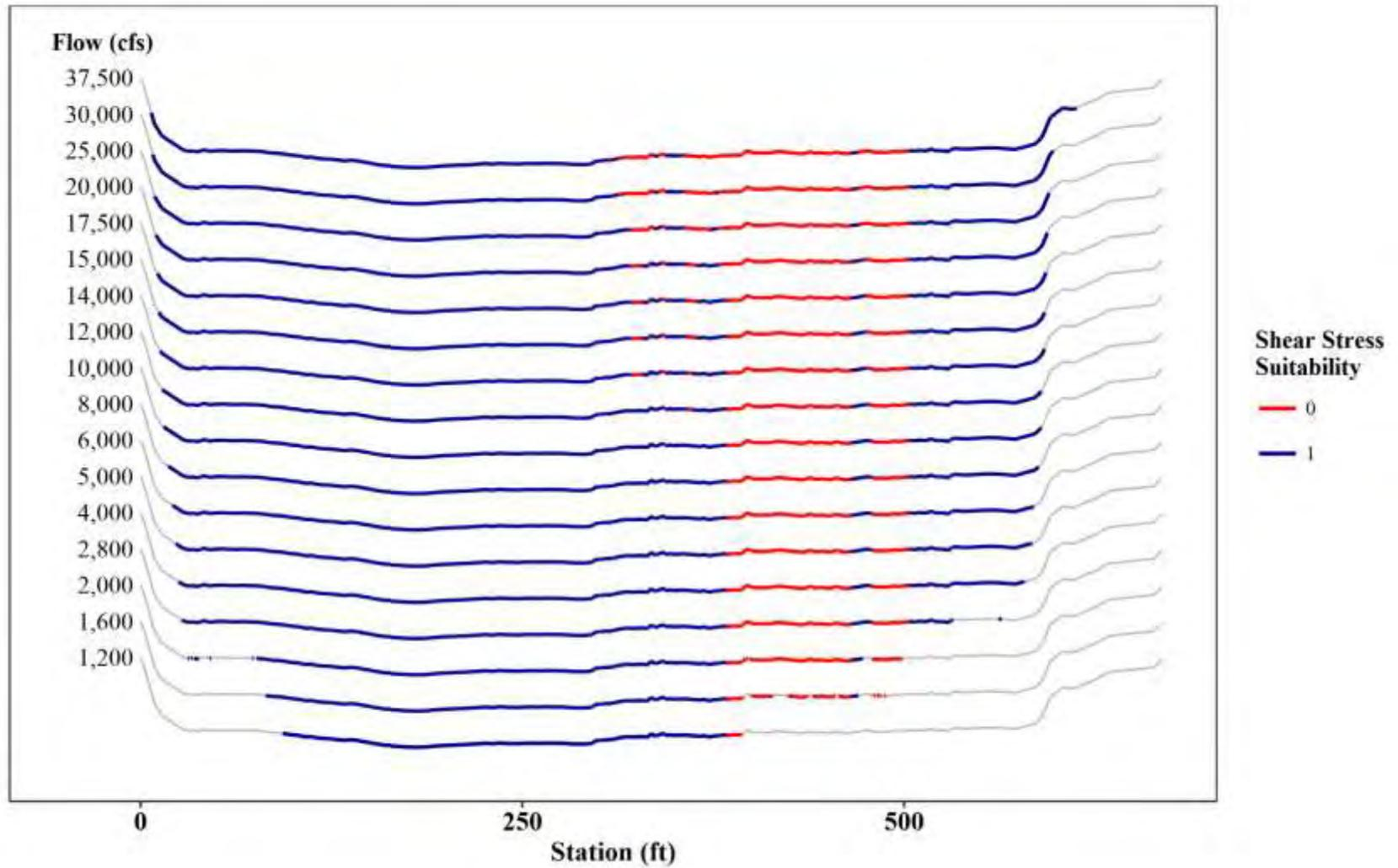
Figure 3.3-5: Shear Stress Mapping at T98 – Adult Yellow Lampmussel
