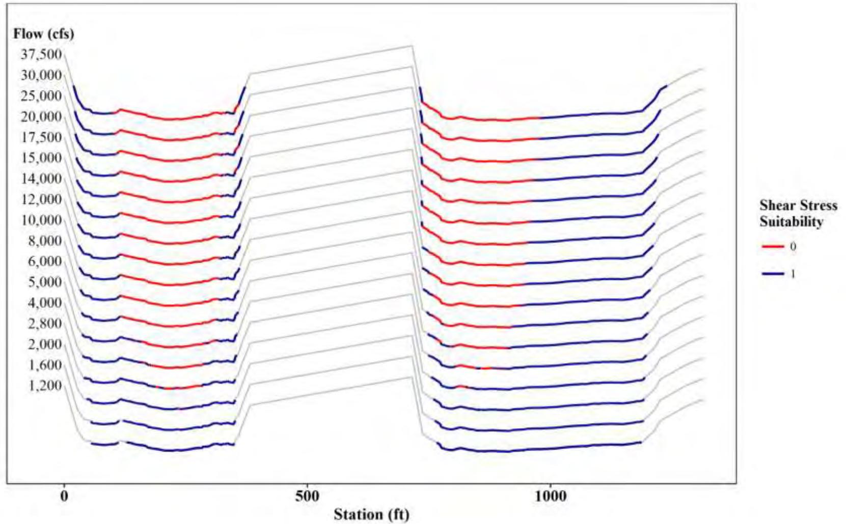
Figure 3.3-22: Shear Stress Mapping at T88 – Juvenile Yellow Lampmussel
