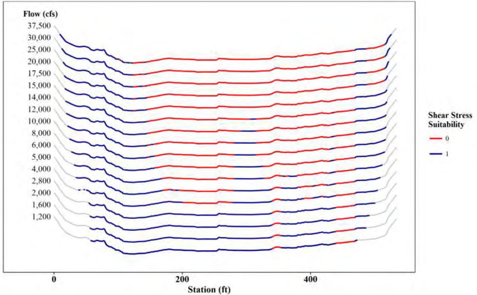
Figure 3.3-10: Shear Stress Mapping at T96 – Juvenile Yellow Lampmussel
