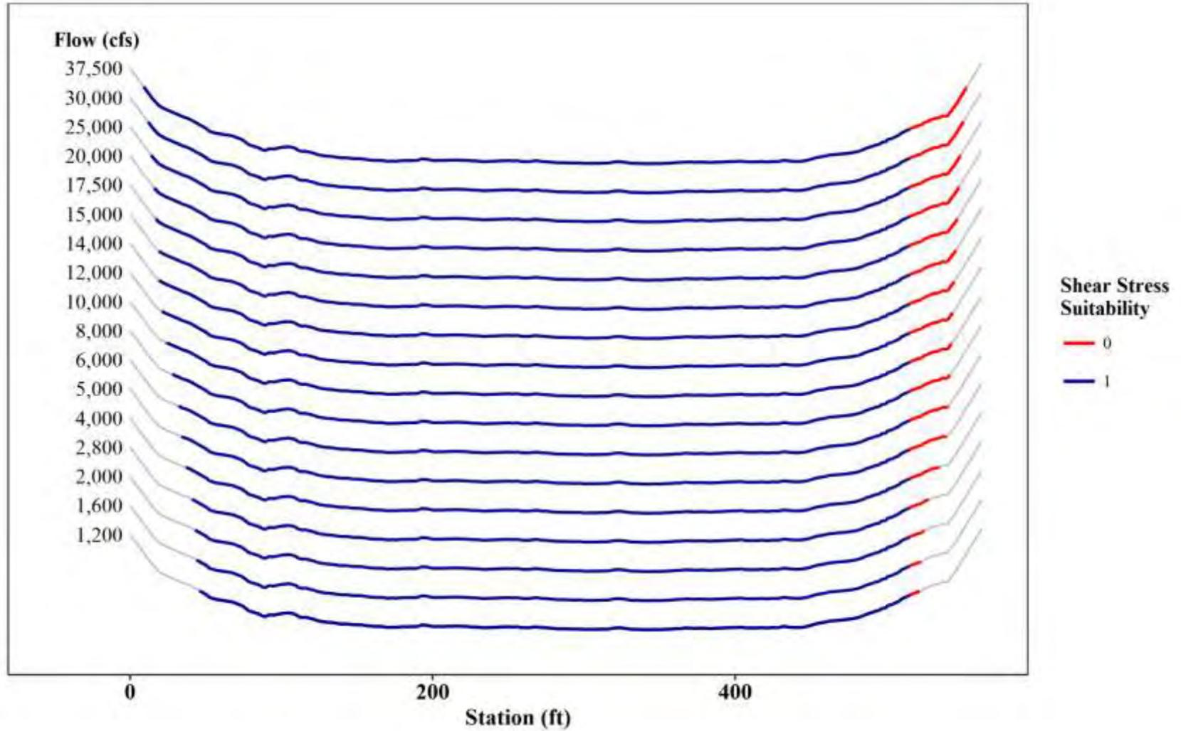
Figure 3.3-15: Shear Stress Mapping at T91 – Adult Yellow Lampmussel
