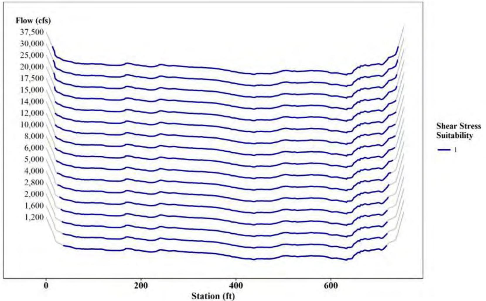
Figure 3.3-23: Shear Stress Mapping at T87 – Adult Yellow Lampmussel
