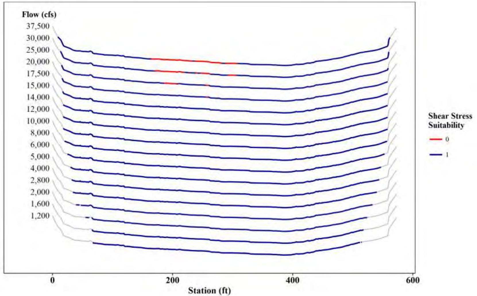
Figure 3.3-1: Shear Stress Mapping at T100 – Adult Yellow Lampmussel
