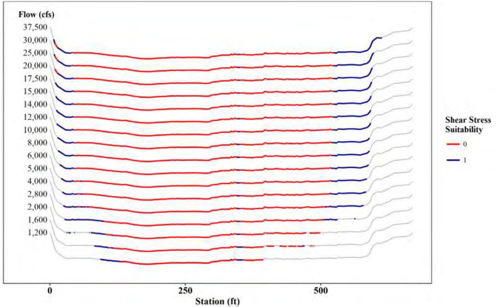
Figure 3.3-6: Shear Stress Mapping at T98 – Juvenile Yellow Lampmussel
