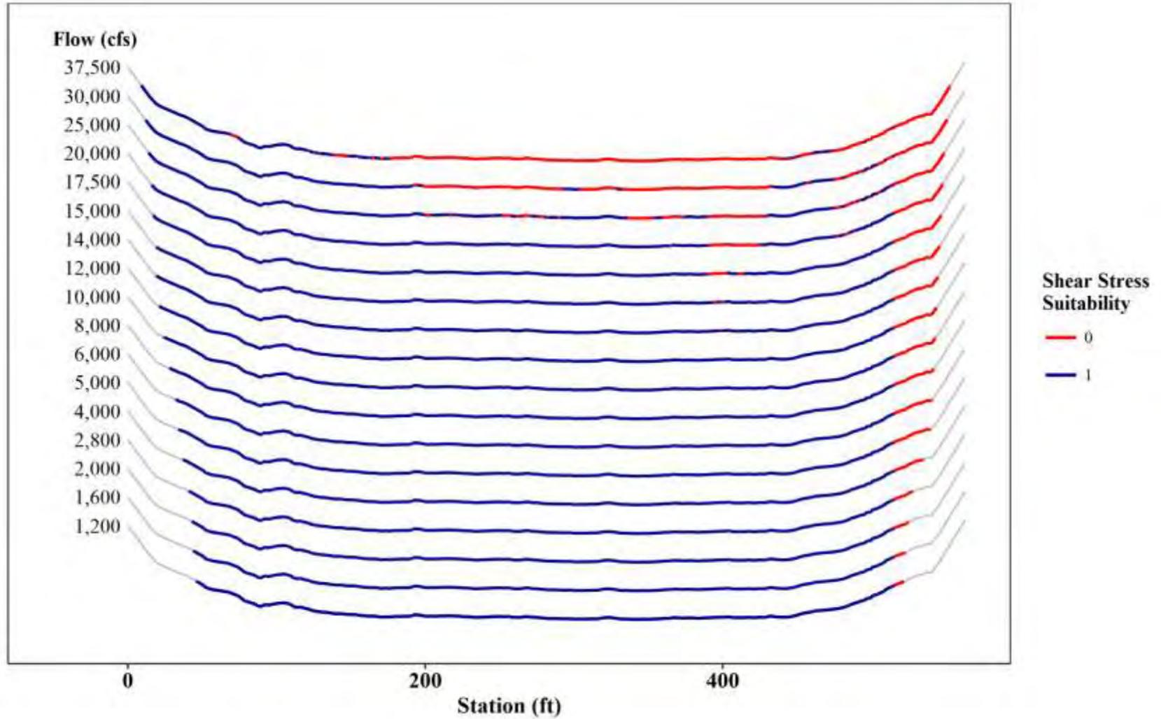
Figure 3.3-16: Shear Stress Mapping at T91 – Juvenile Yellow Lampmussel
