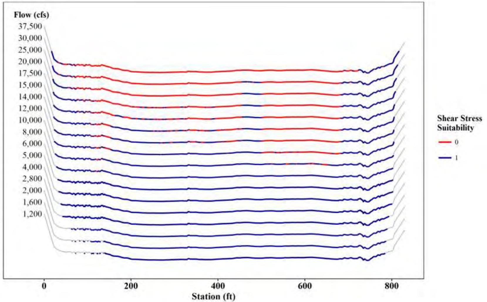
Figure 3.3-20: Shear Stress Mapping at T89 – Juvenile Yellow Lampmussel
