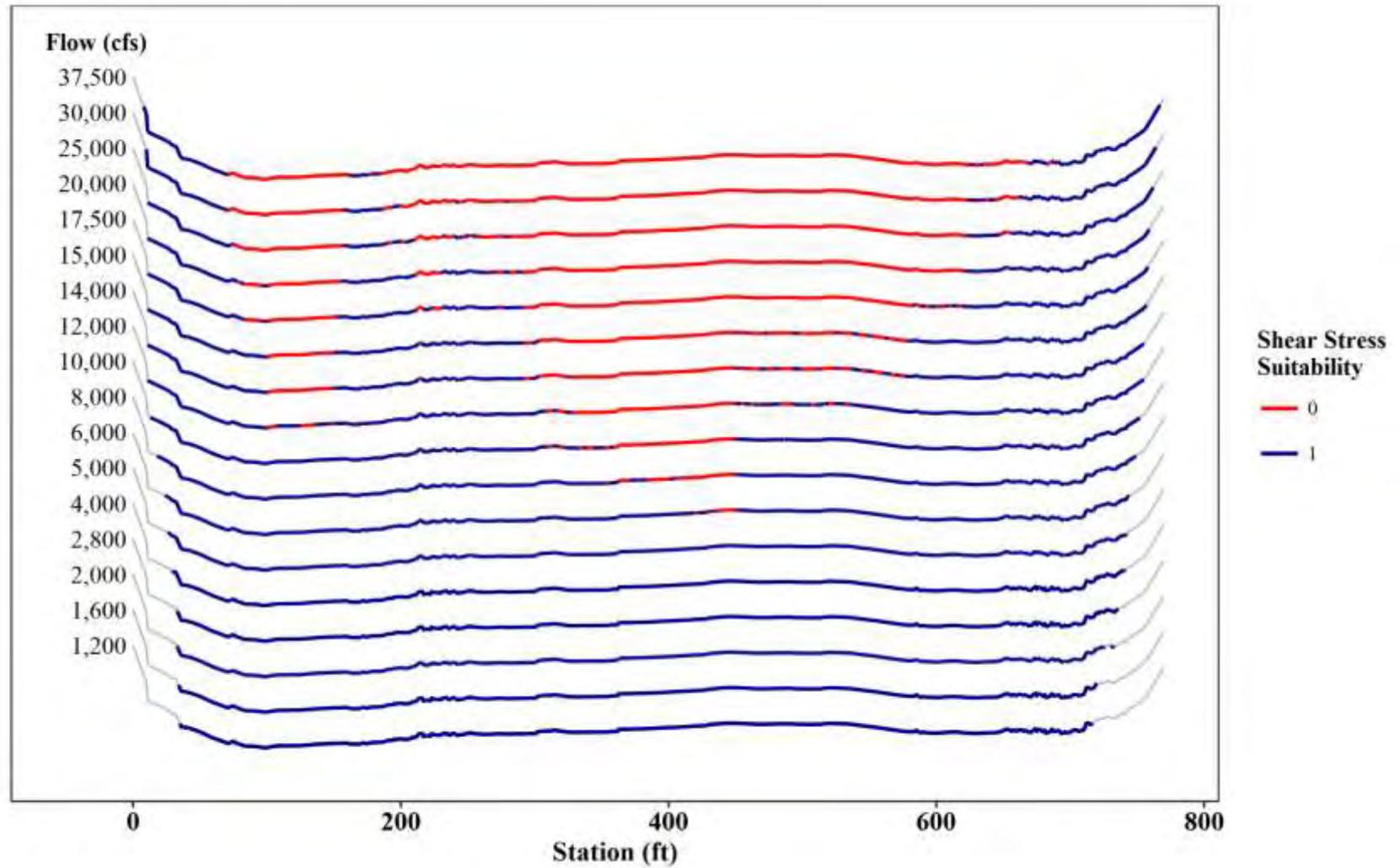
Figure 3.3-14: Shear Stress Mapping at T92 – Juvenile Yellow Lampmussel
