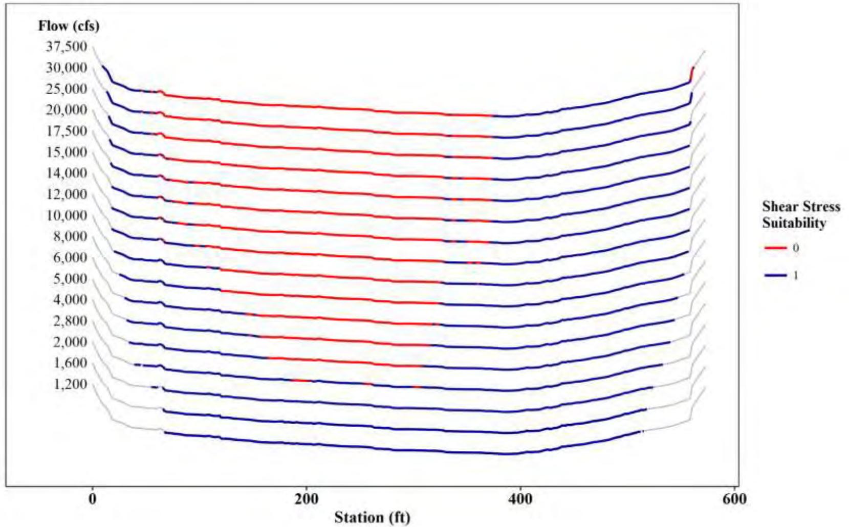
Figure 3.3-2: Shear Stress Mapping at T100 – Juvenile Yellow Lampmussel
