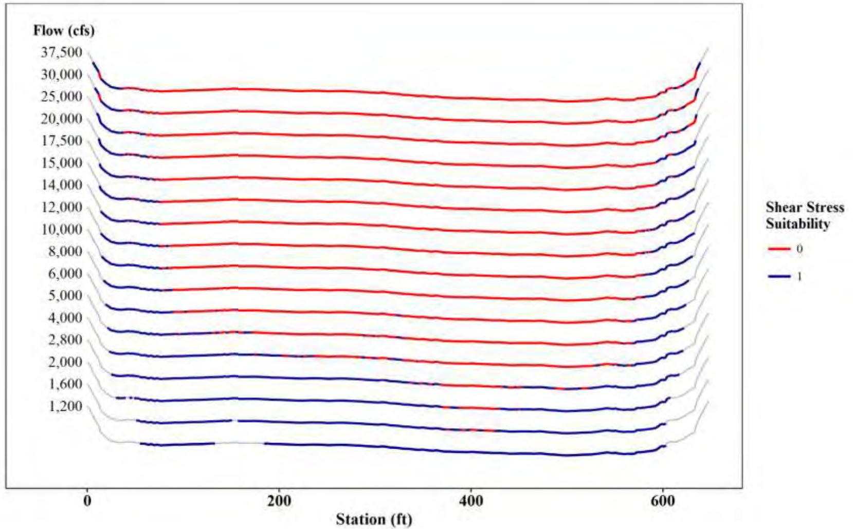
Figure 3.3-12: Shear Stress Mapping at T95 – Juvenile Yellow Lampmussel
