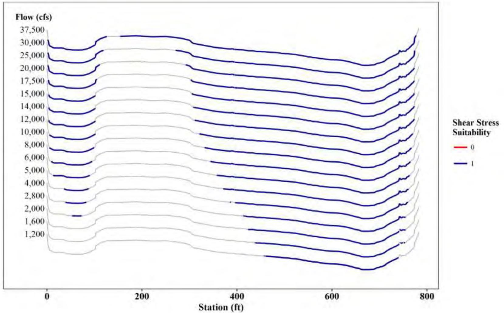
Figure 3.3-3: Shear Stress Mapping at T99 – Adult Yellow Lampmussel
