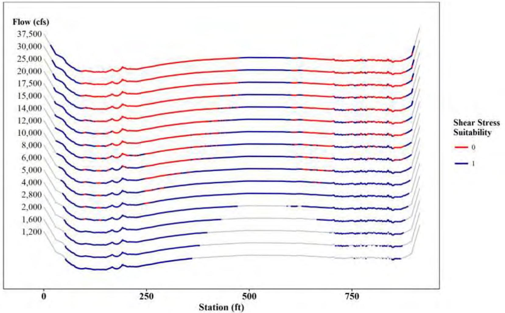
Figure 3.3-18: Shear Stress Mapping at T90 – Juvenile Yellow Lampmussel
