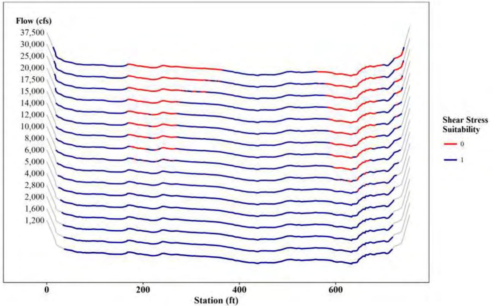
Figure 3.3-24: Shear Stress Mapping at T87 – Juvenile Yellow Lampmussel
