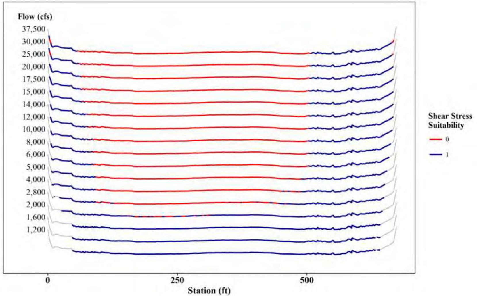
Figure 3.3-8: Shear Stress Mapping at T97 – Juvenile Yellow Lampmussel
