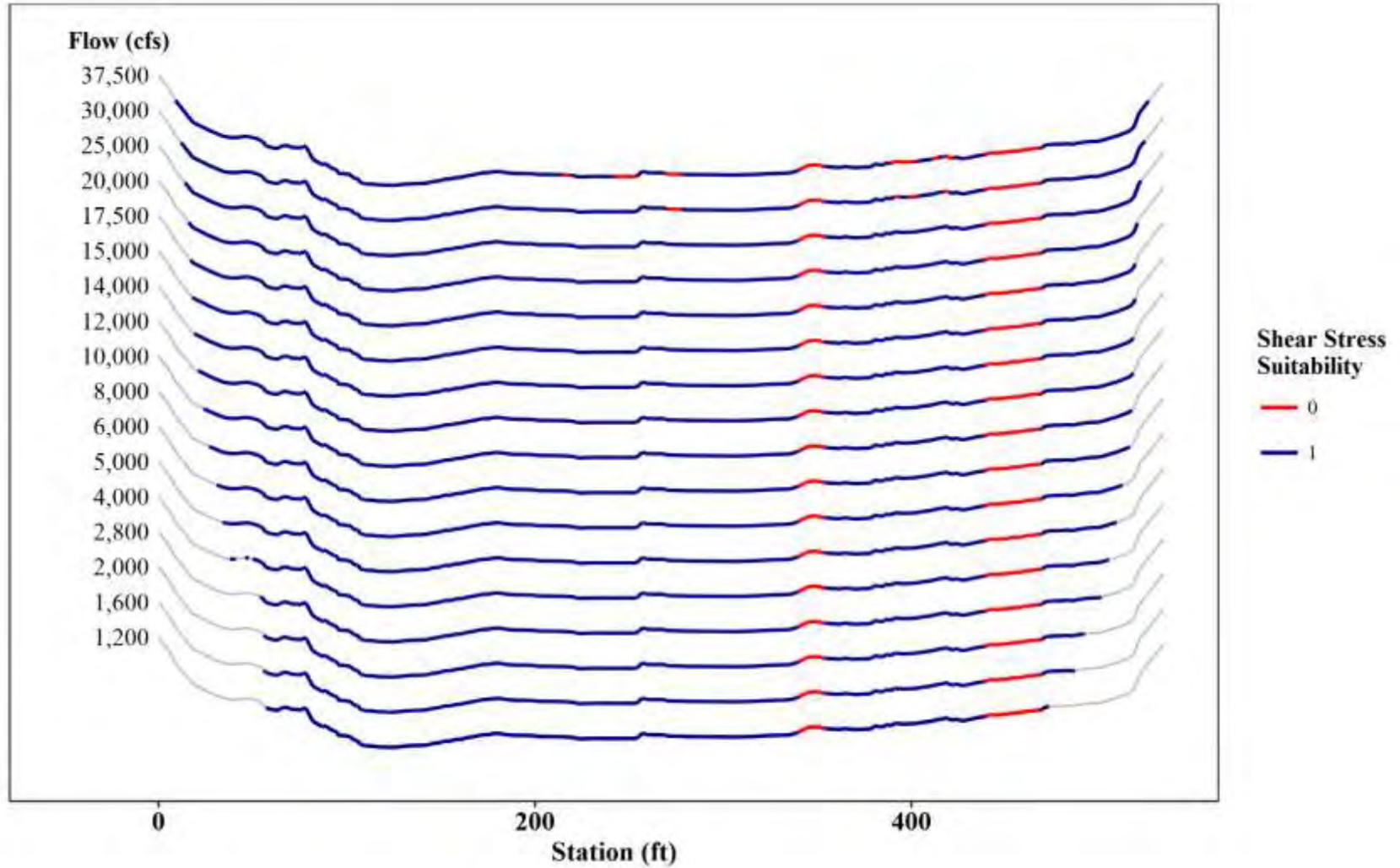
Figure 3.3-9: Shear Stress Mapping at T96 – Adult Yellow Lampmussel
