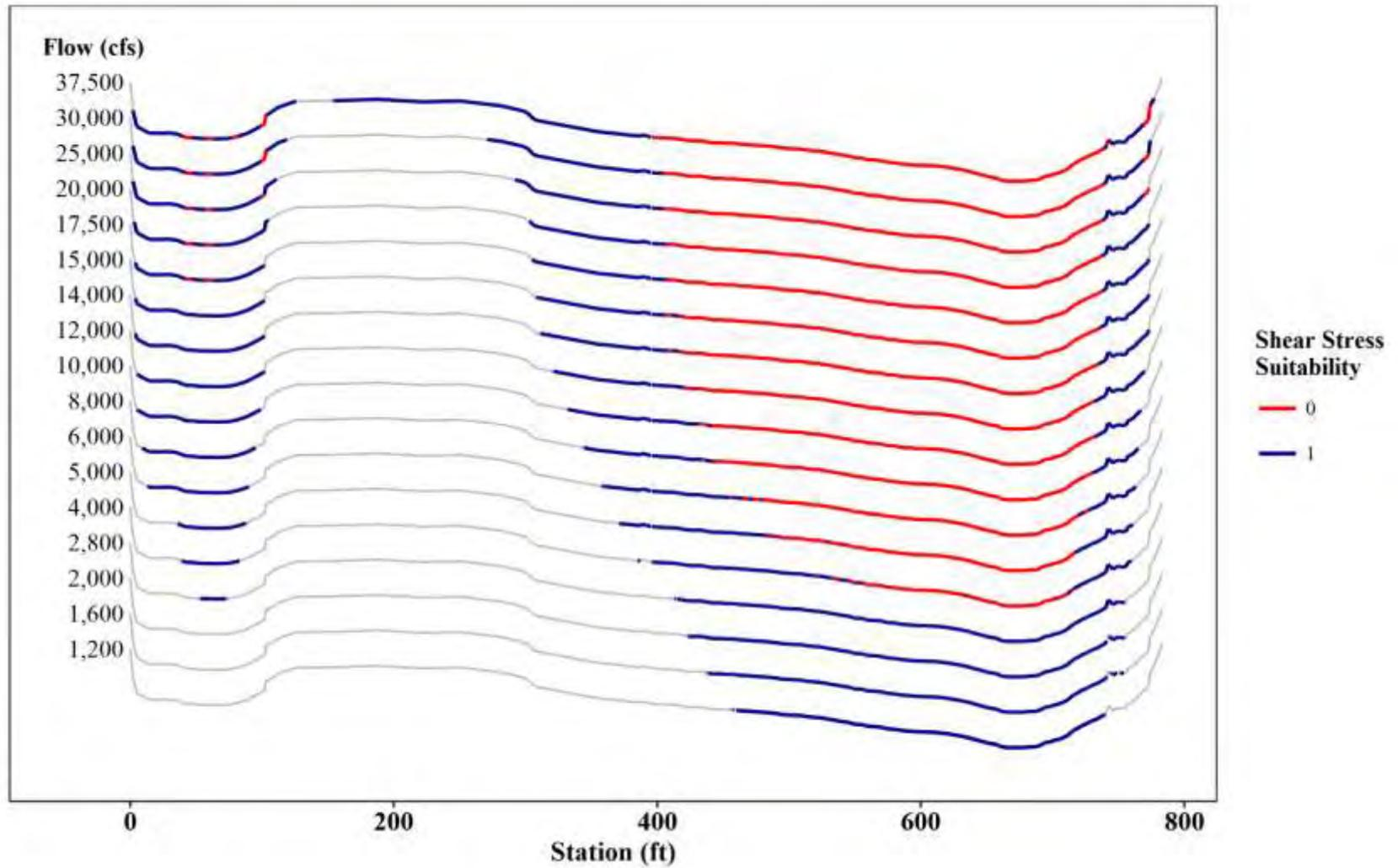
Figure 3.3-4: Shear Stress Mapping at T99 – Juvenile Yellow Lampmussel
