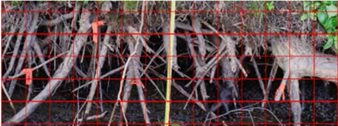
Figure 4.2.7.2-3: Image with 0.1m x 0.1m Grid Superimposed, Ready for Analysis in SigmaScan
