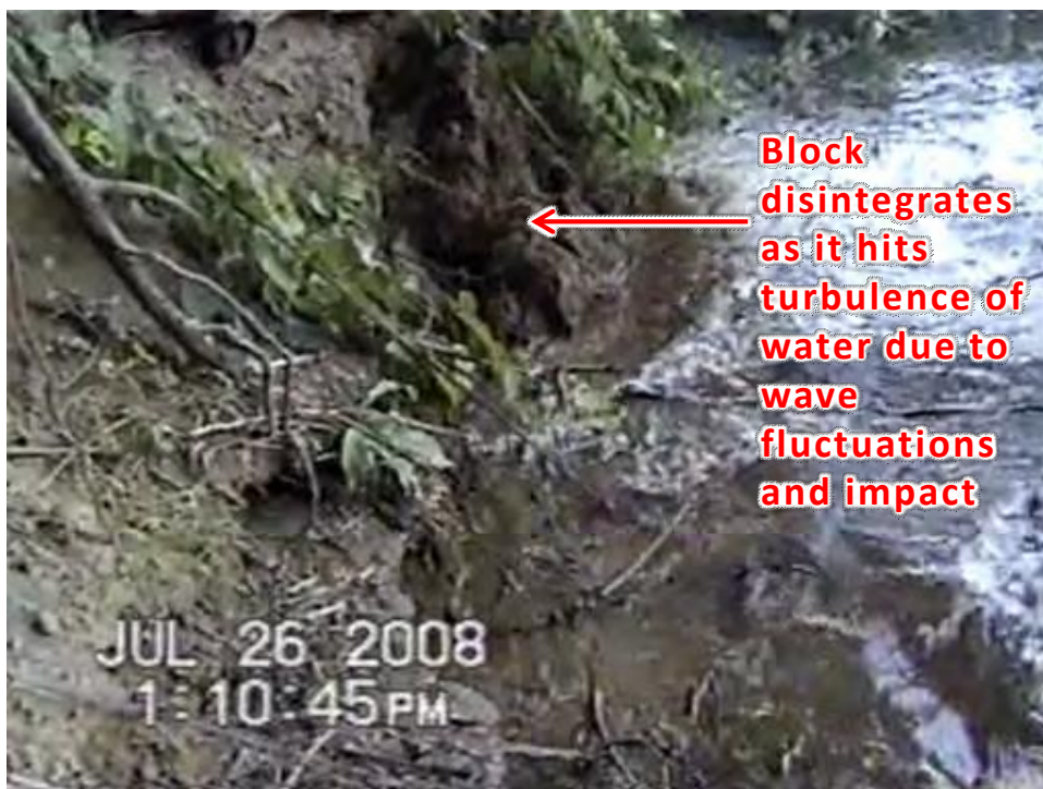
Figure 5.5.3-6b: Boat Wave Erosion Sequence
