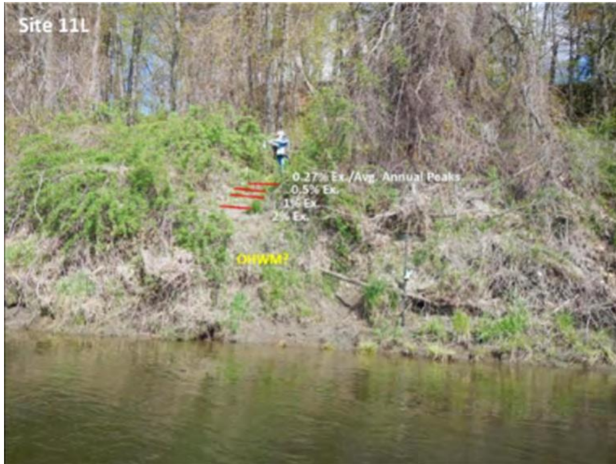
Figure 4.2.4.1-7 Physical characteristics of OHWM at Site 11L
