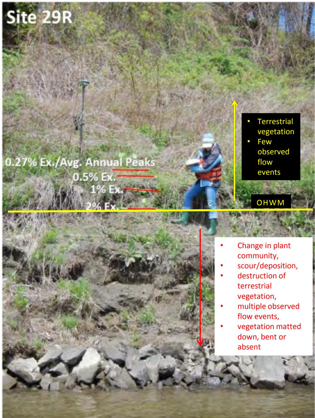
Figure 4.2.4.1-3. Physical characteristics of OHWM at Site 29R
