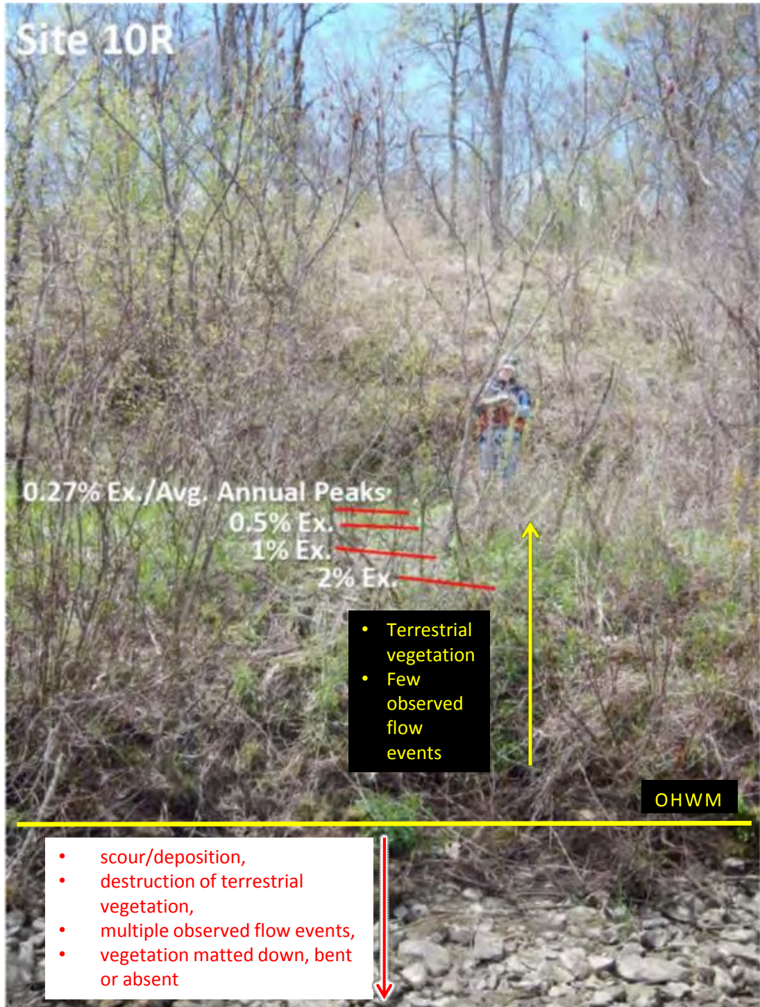
Figure 4.2.4.1-6 Physical characteristics of OHWM at Site 10R
