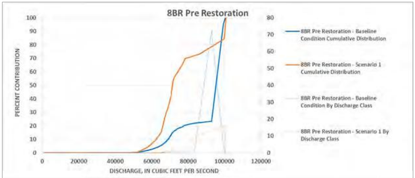
Figure 5.4.3.23-5: Simulated, percent contribution of total erosion by discharge for the Baseline Condition and Scenario 1 at site 8BR for the period 2000-2012
