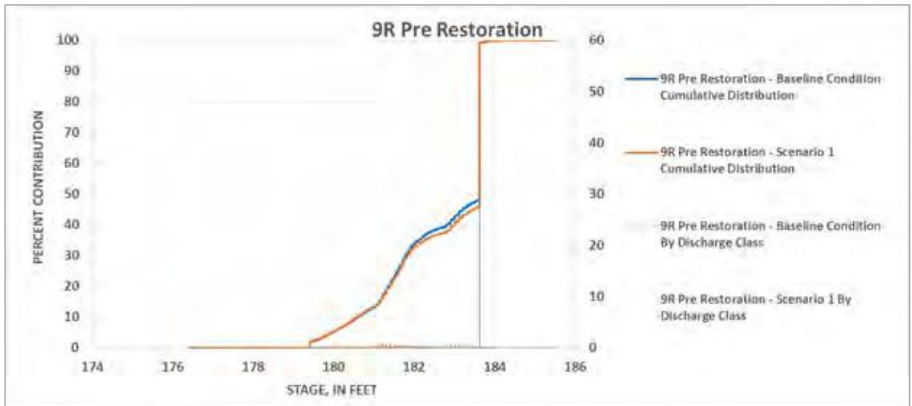
Figure 5.4.3.27-5: Simulated, percent contribution of total erosion by stage for the Baseline Condition and Scenario 1 at site 9R Pre Restoration for the period 2000-2008. As no stage-discharge relationship could be developed, stage was used
