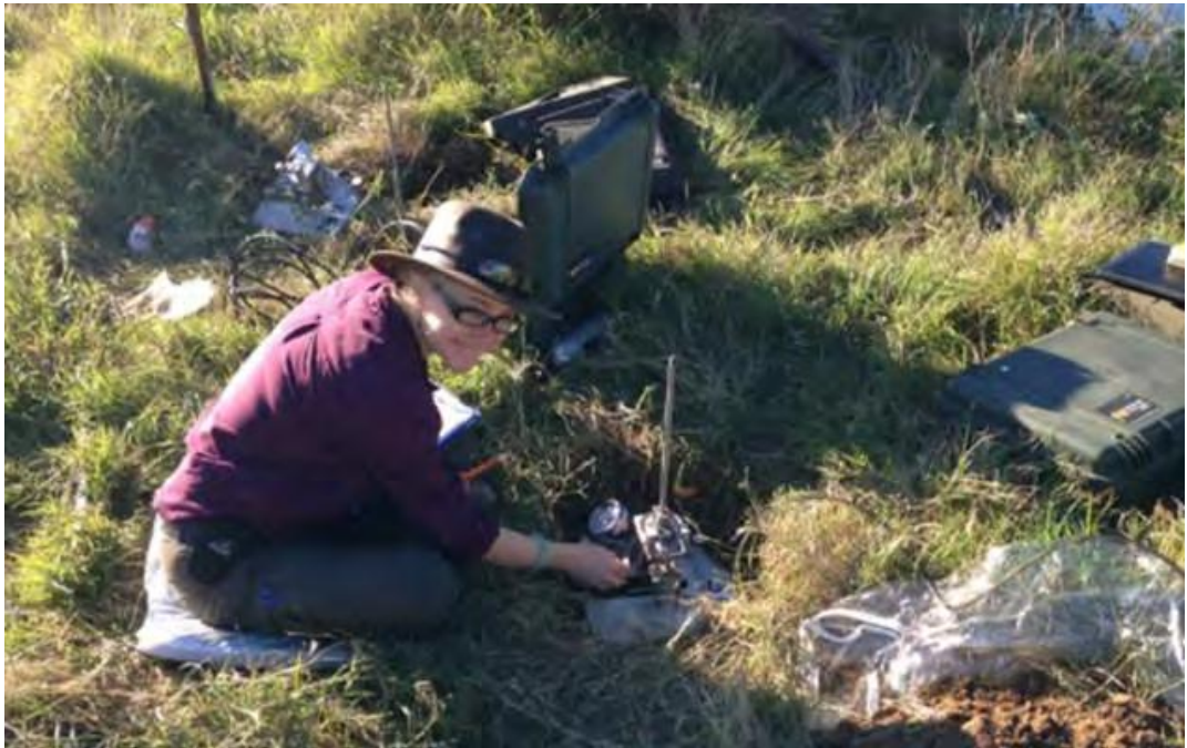
Figure 4.2.6.1-2: Conducting a Borehole Shear Test (BST)
