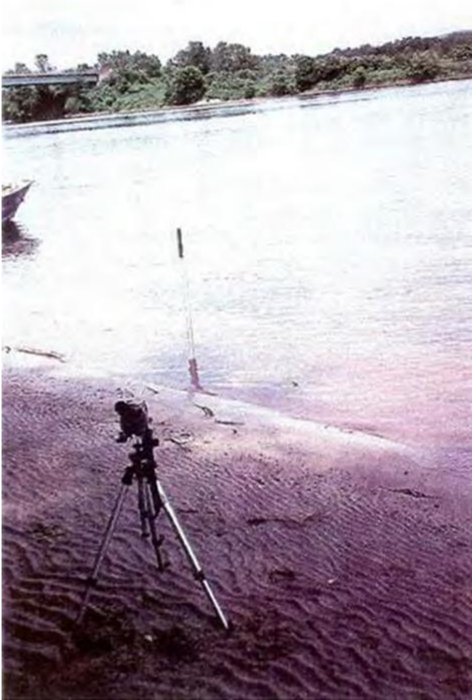
Figure 5.5.3-1: Video Camera and Temporary Staff Gage
