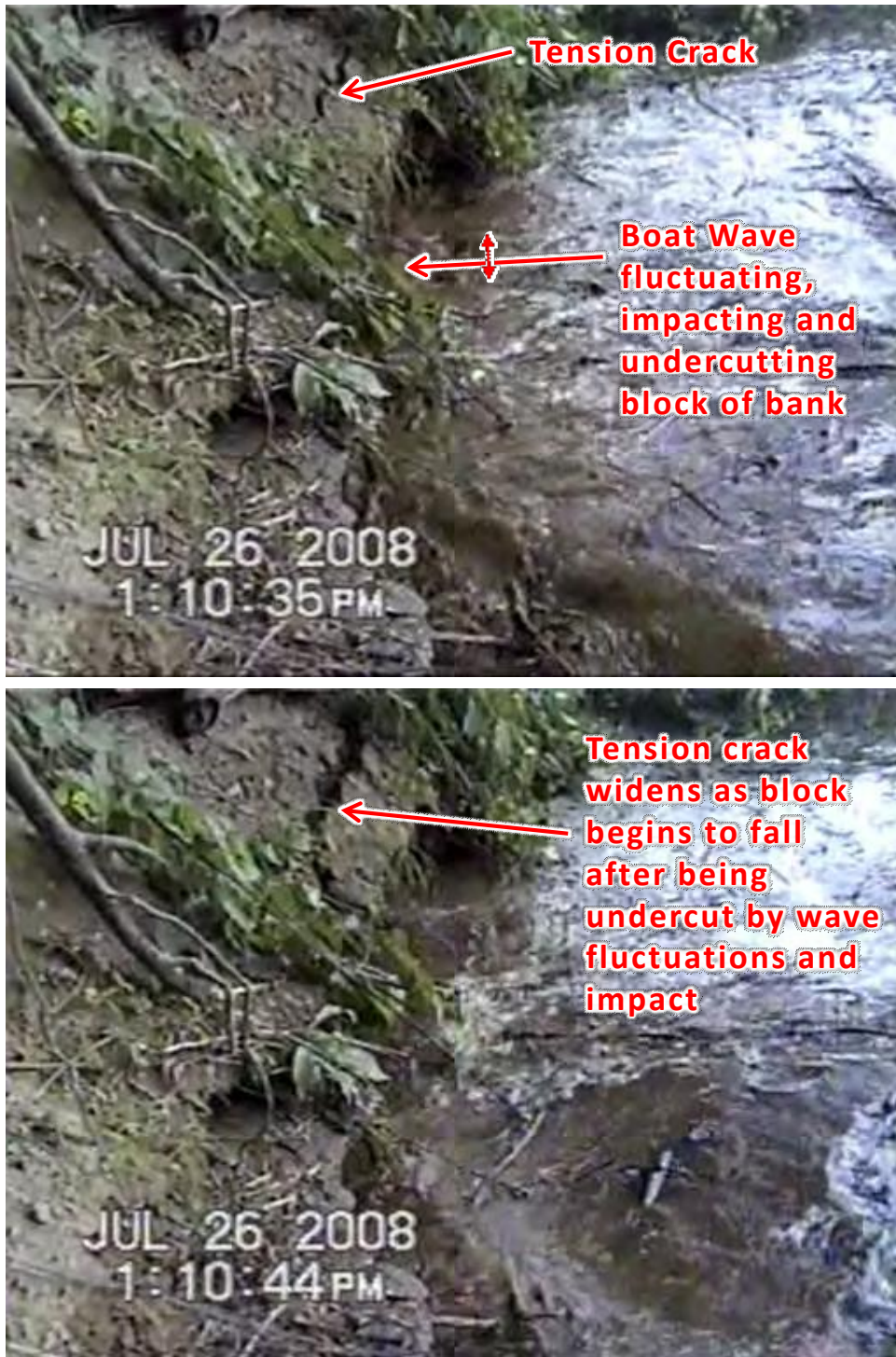
Figure 5.5.3-6a: Boat Wave Erosion Sequence
