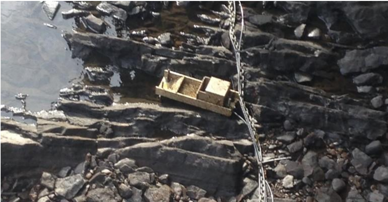
Figure 3.1.2-2: Custom Leveling Mount used to Position the Split Beam Transducers on the Bottom of the Cabot Power Canal.
