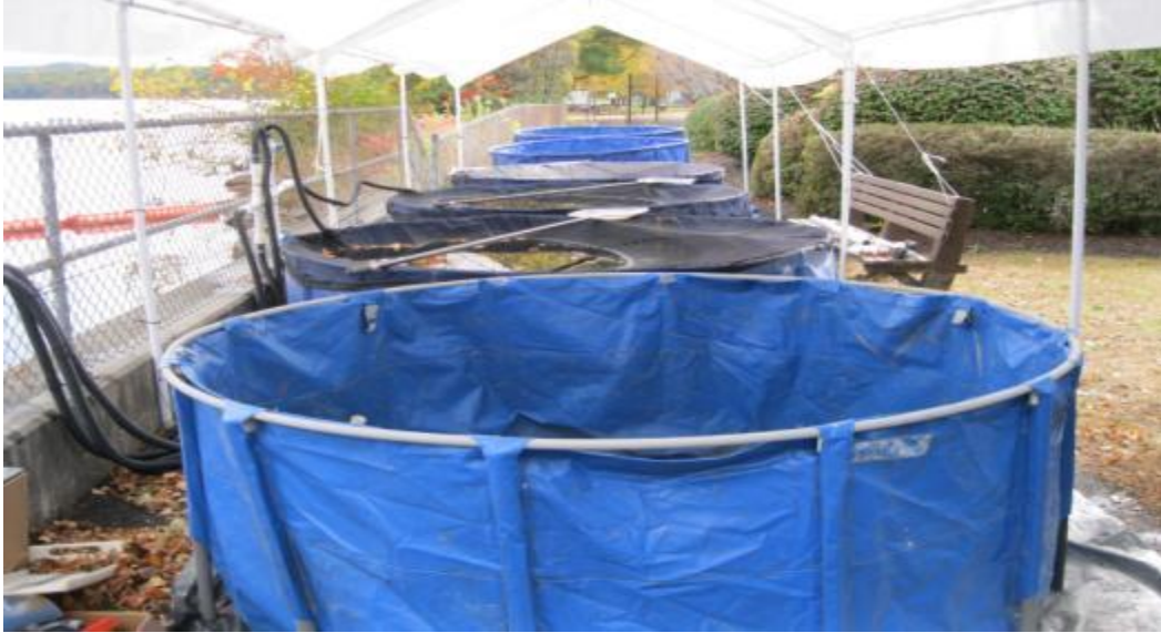
Figure 4-14 Fish holding tanks continuously supplied with ambient river water by two redundant pump systems connected to different electrical circuits, and were numbered to clarify test dates.
