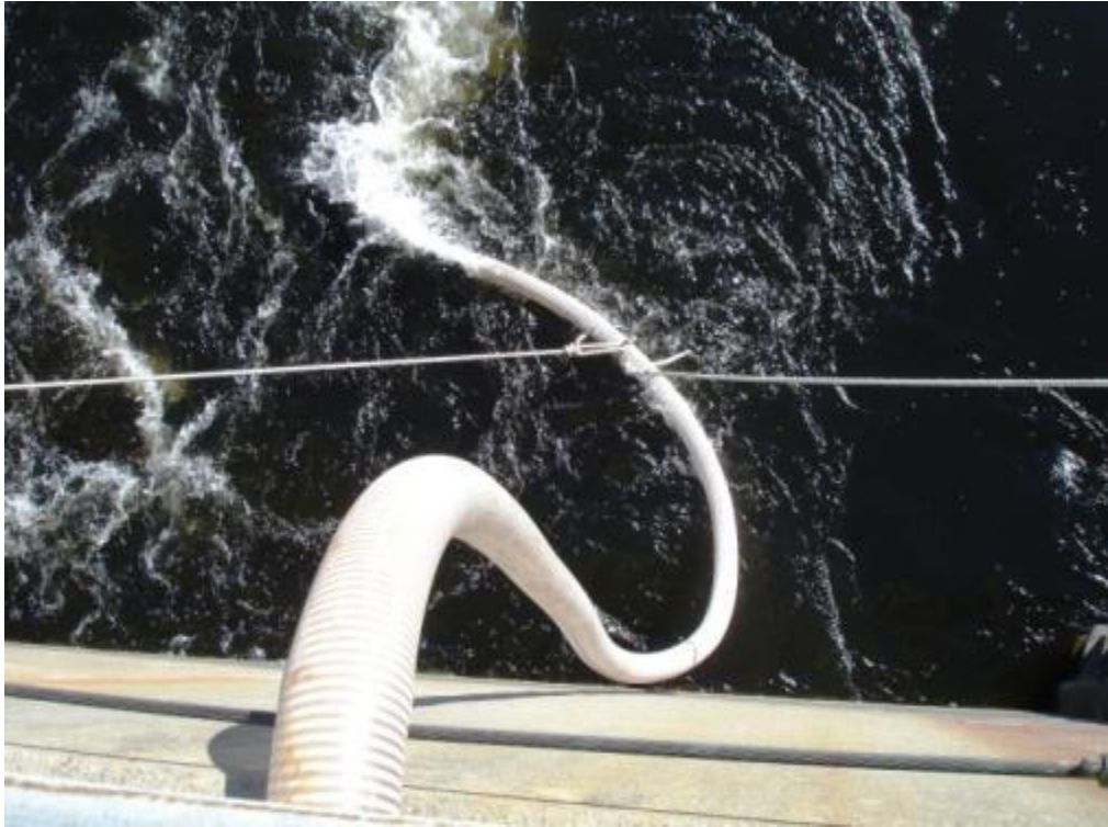
Figure 4-10 The induction apparatus connected to 4-inch diameter hoses which allowed the shad to pass to the desired release points.
