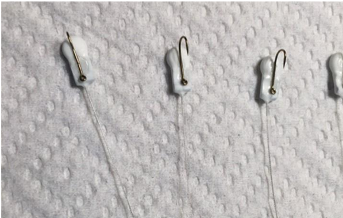
Figure 3.2.2-2. Lotek NanoTag Series Model NTQ-1 affixed to a No. 16 Dry Fly Fishing Hook
