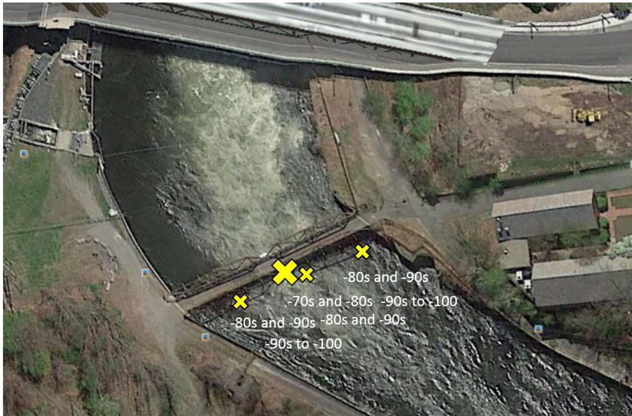
Figure A-8: The large yellow X marks the approximate placement of the yagi antenna and the Orion receiver used to detect fish moving in the canal at River Mile 122. The small Xs mark the approximate locations of the three in-water droppers used at this location to assist with monitoring the passage of downstream eel as well as juvenile shad. The radio test tag produced power levels ranging from -70s to -100 db with highest powers located near yagi antenna and attenuating farther out from the antenna.
