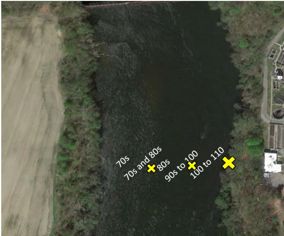
Figure A-1: The large yellow X marks the approximate placement of the yagi antenna and the Lotek receiver used to detect fish moving across the width of the river at River Mile 119.5. The smaller X's mark the approximate locations of the two in-water droppers used at this location to assist with monitoring the passage of juvenile shad. The radio test tag produced power levels ranging from 70s to 110 db with highest powers located near the bank of the river closest to the yagi antennas and attenuating slightly toward the far bank.
