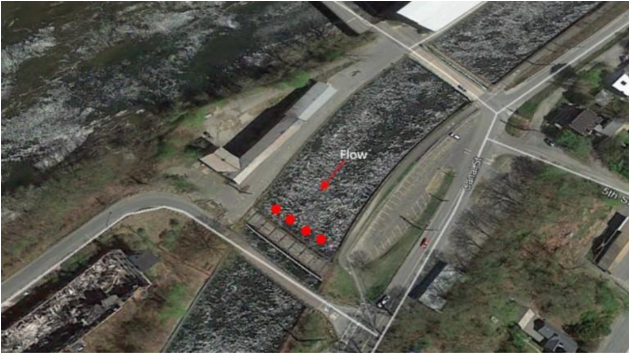
Figure 3.1.2-1: Location of the Four Split Beam Transducers (in red, not to scale) used to Monitor Juvenile Shad as they Migrate through the Turners Falls Power Canal
