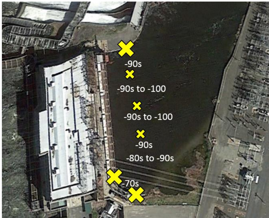
Figure A-3: The large yellow Xs mark the approximate placement of the yagi antennas, the dipole antenna and the Orion receivers used to detect fish moving across the Cabot Station Forebay at River Mile 120. The small Xs mark the approximate locations of the four in-water droppers used at this location to assist with monitoring the passage of downstream eel as well as juvenile shad. The radio test tag produced power levels ranging from -70s to 100 db with highest powers located near the bank of the river closest to the yagi antennas and attenuating slightly toward the far bank.
