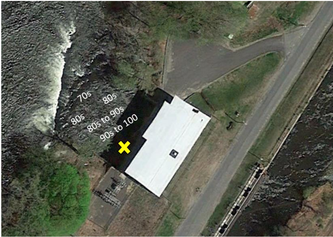
Figure A-5: The large yellow X marks the approximate placement of the yagi antenna and the Lotek receiver used to detect fish within the Station No.1 tailrace at River Mile 121. The radio test tag produced power levels ranging from -70 to -90 with highest powers located closest to the yagi antennas and attenuated in the middle of the Station No. 1 Tailrace.
