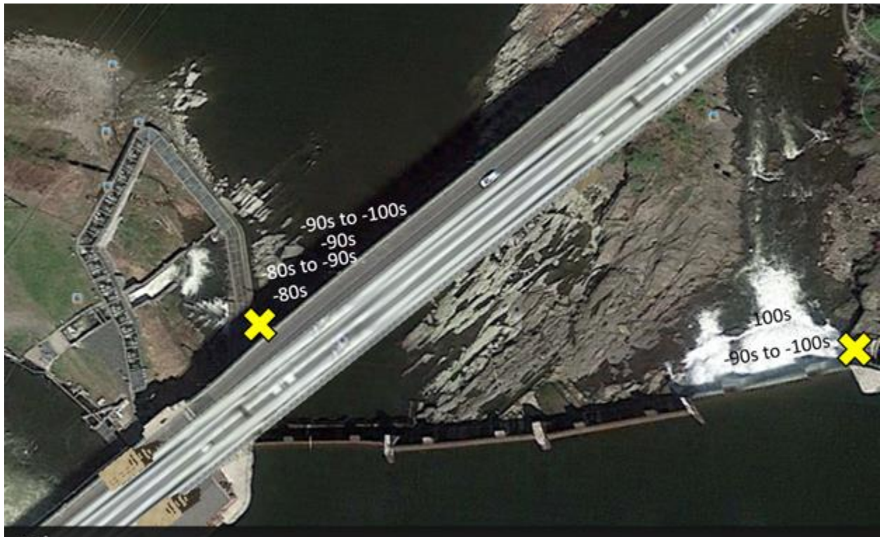
Figure A-6: The large yellow X marks the approximate placement of the yagi antennas and the Orion receivers used to detect fish below the Turners Falls dam (river left) and below Bascule Gate 4 at River Mile 122. The radio test tag produced power levels below the dam at river left ranging from -80 to -100s with highest powers located closest to the yagi antennas and attenuated farther out from the antenna. Below bascule gate 4, power levels ranged from -90s to -100s.
