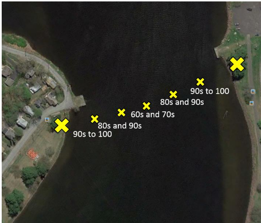
Figure A-10: The large yellow Xs mark the approximate placement of the yagi antennas and the Lotek receivers used to detect fish in the Turners Falls Impoundment at River Mile 122. The small Xs mark the approximate locations of the five in-water droppers used at this location to assist with monitoring the passage of downstream eel as well as juvenile shad. The radio test tag produced power levels ranging from 60 to 100 db with highest powers located near yagi antennas and attenuating farther out from the antennas.
