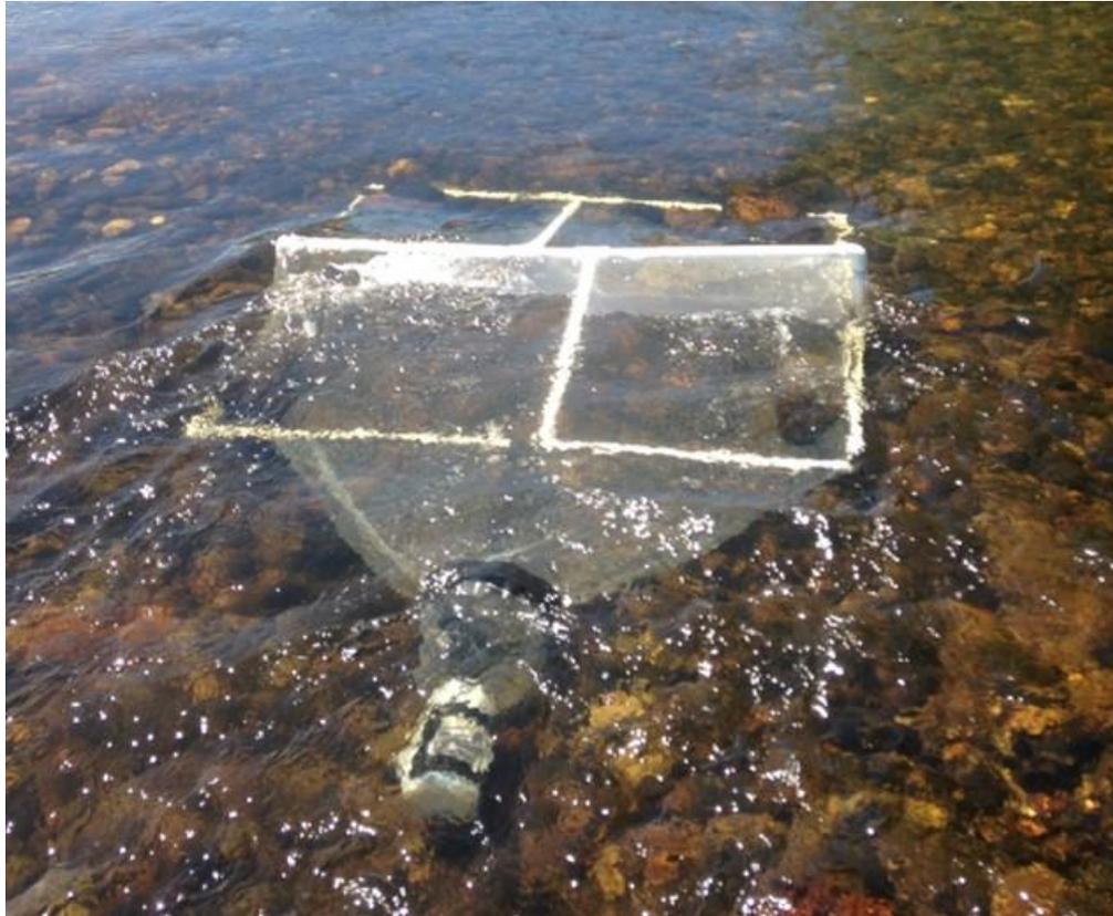
**Figure 3.3-1: Lamprey Redd Cap: 4x4 ft, Weighted PVC Framed Collection Net (1 mm Mesh) Funneling into a Collection Jar.**
