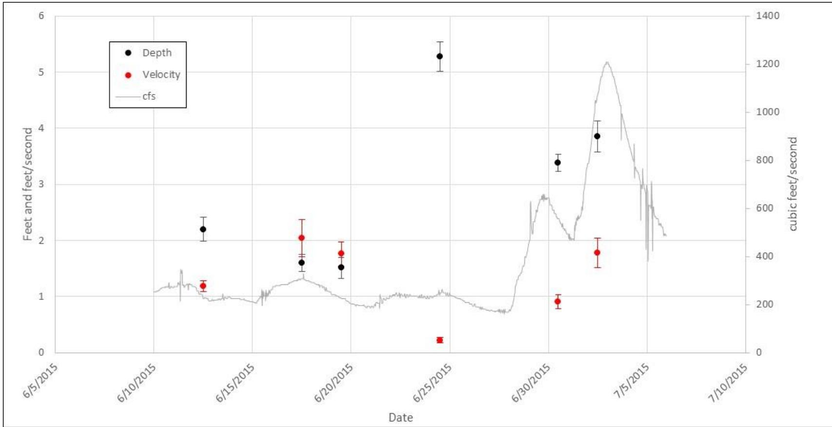
**Figure 4.5-2: Ashuelot River Discharge (cfs) During Lamprey Sampling Period (6/12/15 to 7/6/15) with mean daily velocity (fps) (+/- SD) and mean daily depth (ft) (+/- SD) Measurements of the 11 redds monitored**
