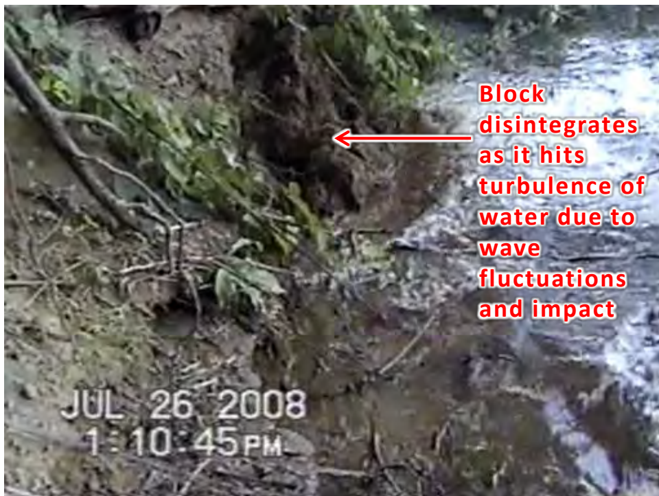
Figure 5.5.3-6b: Boat Wave Erosion Sequence
