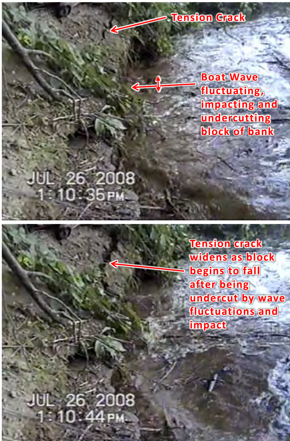
Figure 5.5.3-6a: Boat Wave Erosion Sequence
