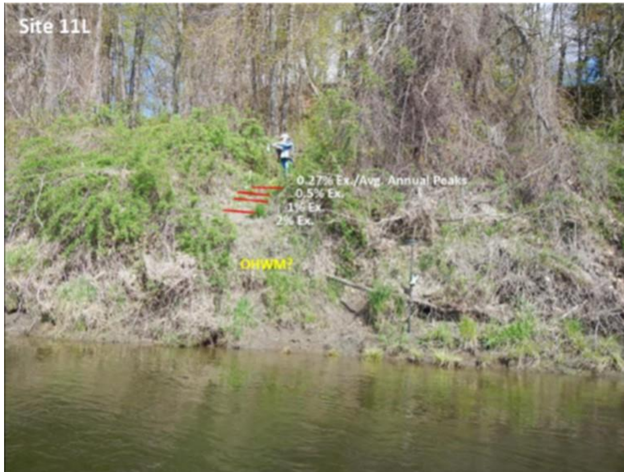
Figure 4.2.4.1-7 Physical characteristics of OHWM at Site 11L
