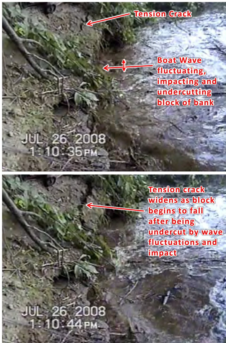
Figure 5.5.3-6a: Boat Wave Erosion Sequence
