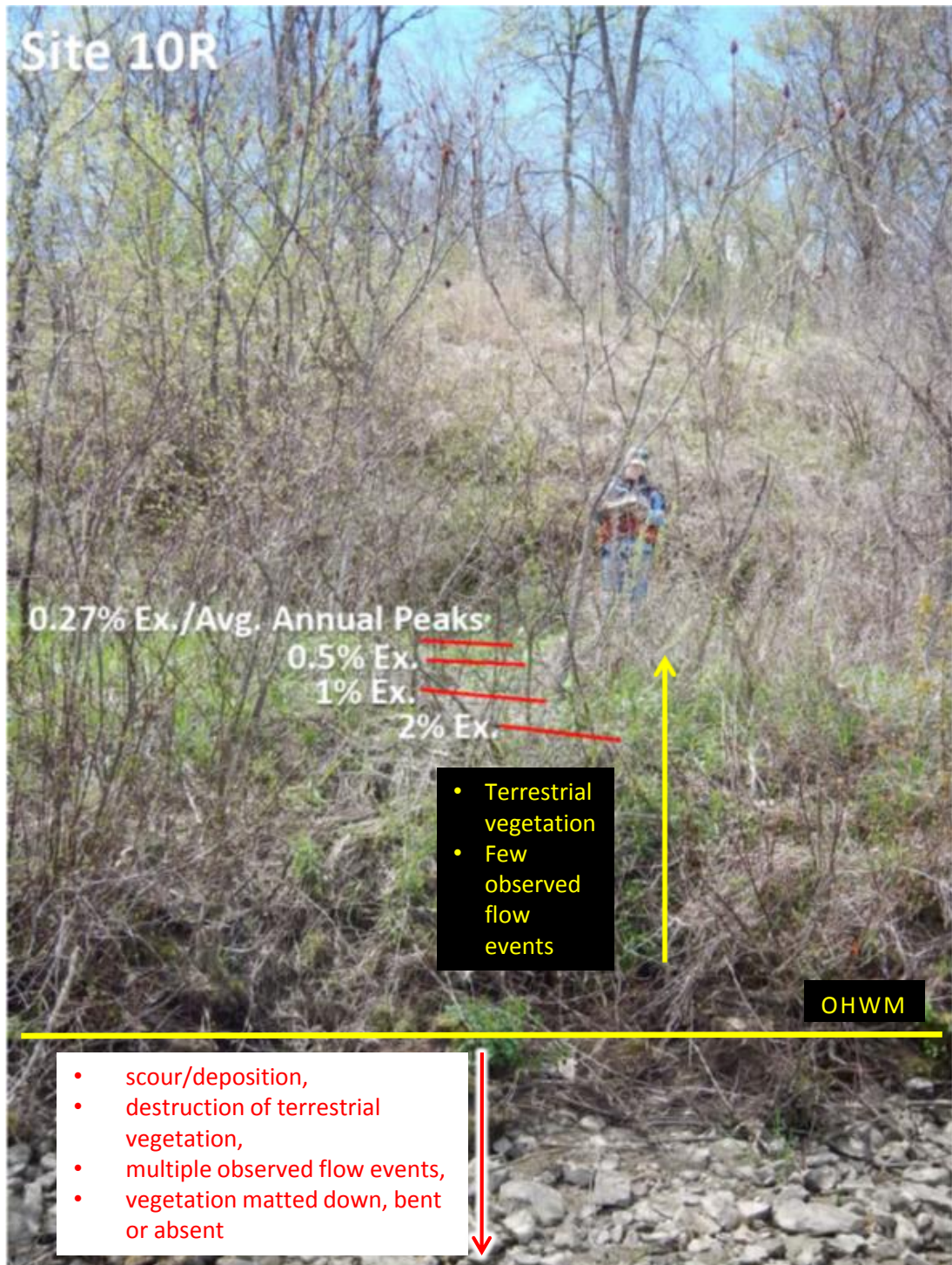
Figure 4.2.4.1-6 Physical characteristics of OHWM at Site 10R
