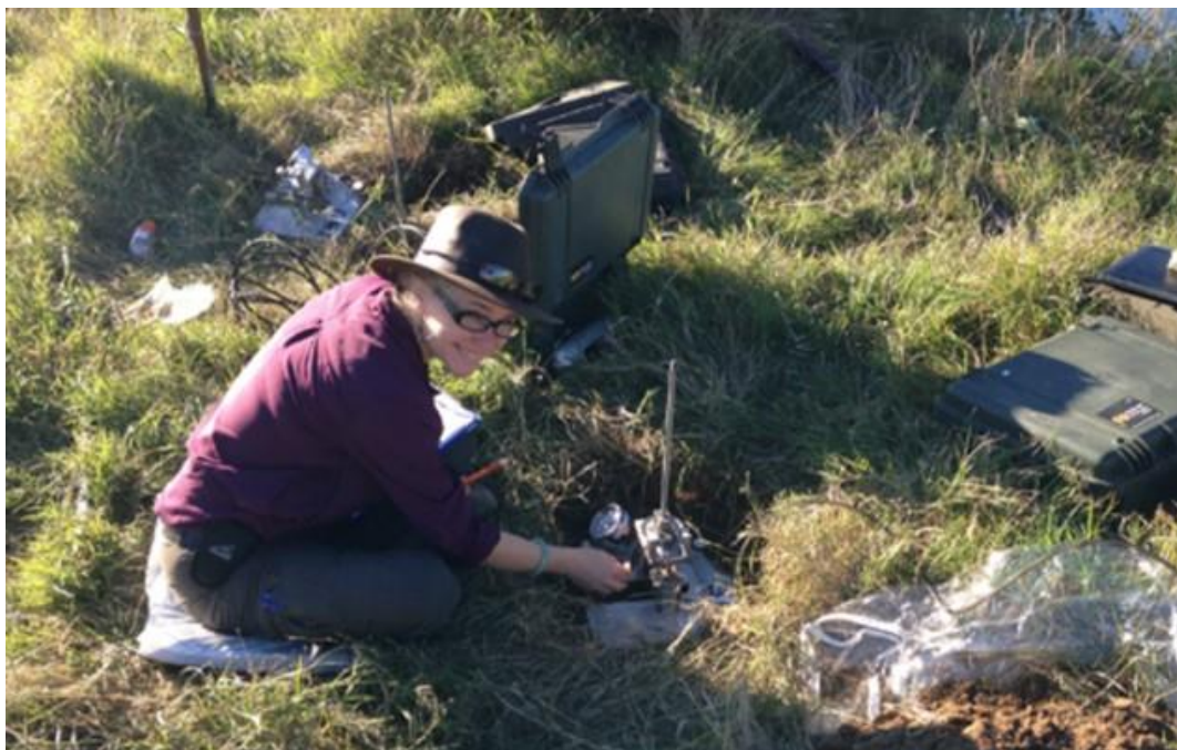
Figure 4.2.6.1-2: Conducting a Borehole Shear Test (BST)
