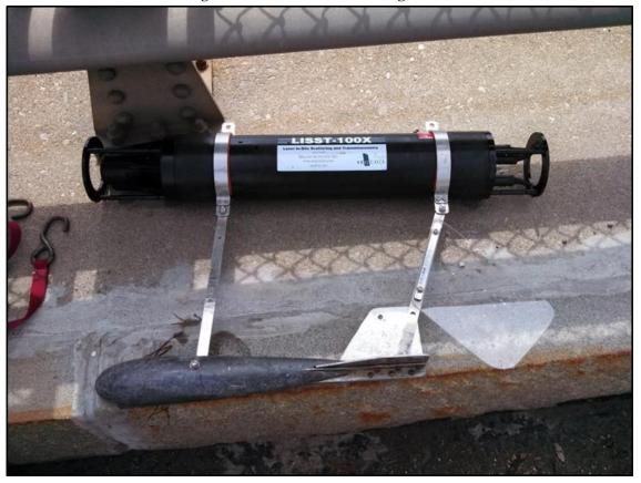
Figure 2.2.1-6 LISST-100X Configuration
