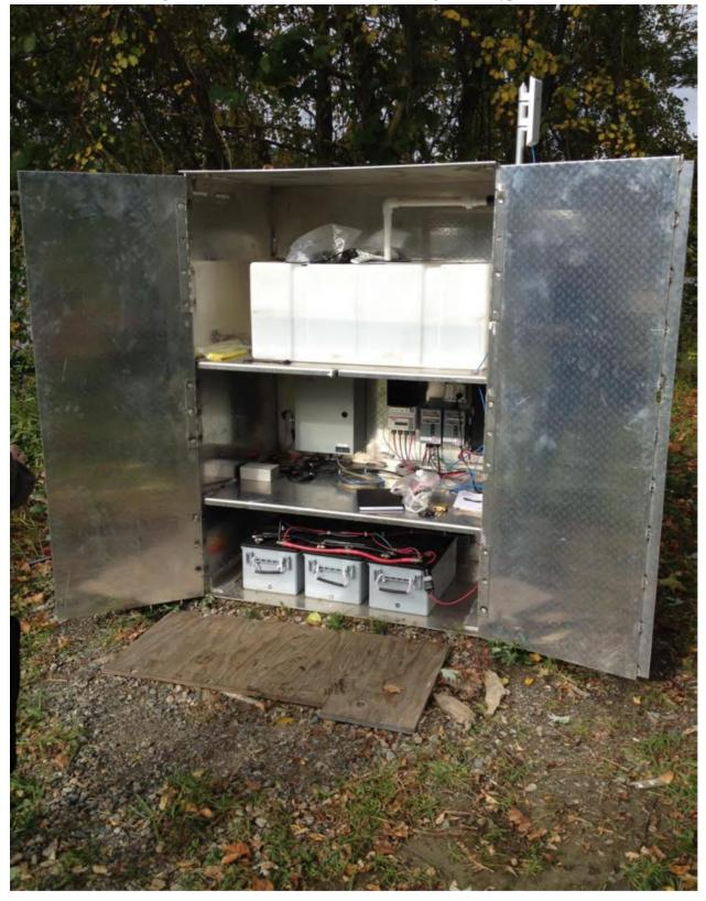
Figure 2.2.1-3 LISST-HYDRO Cabinet Configuration (typical)
