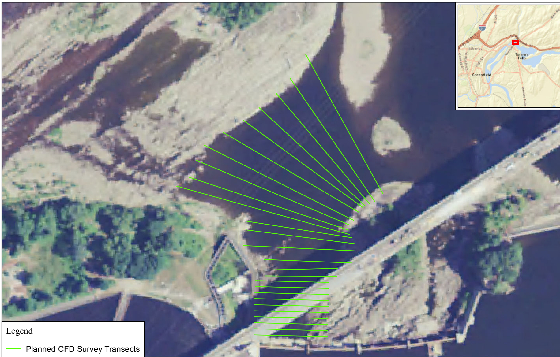
Figure 4 - Planned Bathymetry and Velocity CFD Transects at the Spillway Fishway.
