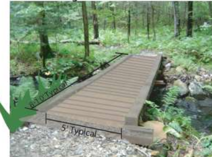
Standard Repair Diagram: Elevated Bridge
