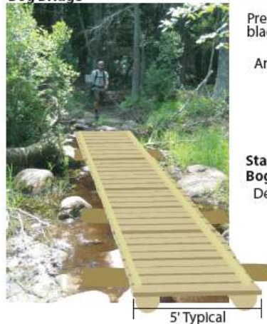
Standard Repair Diagram: Bog Bridge
